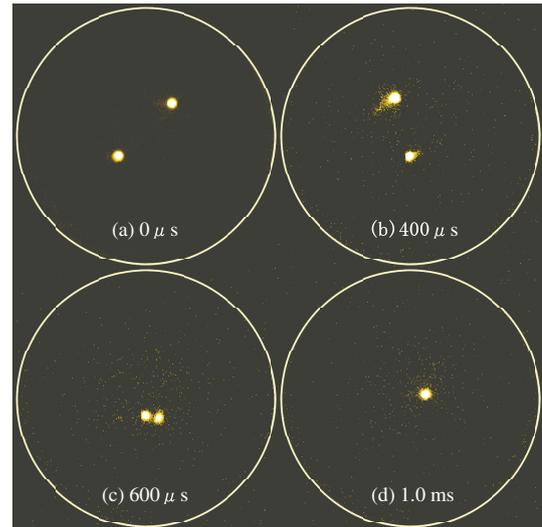
Fig. 2 A typical set of pictures that shows how a single  $\text{e}^-$  plasma is formed from several  $\text{e}^-$  beams on BX-U. Through a self-organization process, those beams are merged together completely.
