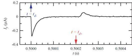
Fig. 4 A typical waveform of  $I_f$ . The data is smoothed. At  $t = t_{d-}$ , the  $e^-$  plasma is flowing out, while the  $Li^+$  plasma is extracted at  $t = t_{d+}$ .
