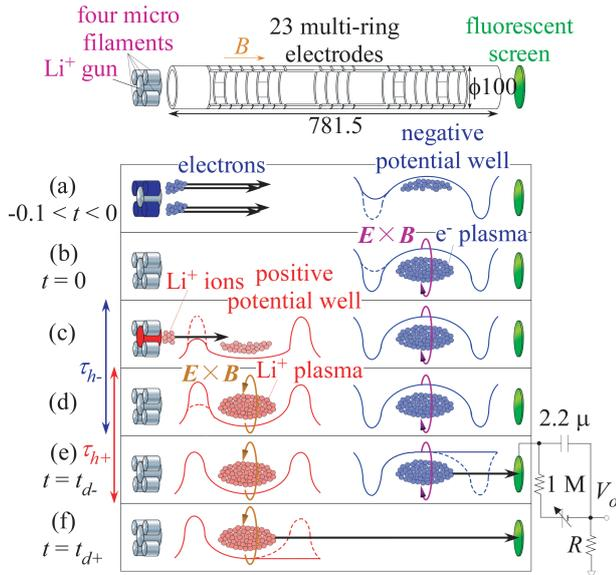
Fig. 1 A schematic diagram of the experiment producing and confining both lithium ion ( $\text{Li}^+$ ) and electron ( $\text{e}^-$ ) plasmas simultaneously.
