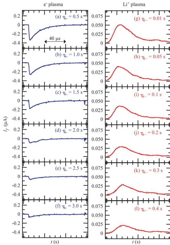
Fig. 3 A typical set of time histories of  $I_f$  measured by the end-on collector for cases where either (a) - (f) an  $e^-$  or (g) - (l) a  $Li^+$  plasma is confined independently. As recognized, successful confinements of both non-neutral plasmas are certainly realized.
