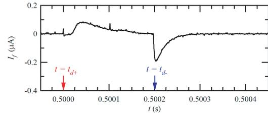
Fig. 5 A typical waveform of  $I_f$ . The data is smoothed. Contrary to the case in Fig. 4, the  $Li^+$  plasma is firstly extracted at  $t = t_{d+}$ , and subsequently, the  $e^-$  plasma is flowing out at  $t = t_{d-}$ .
