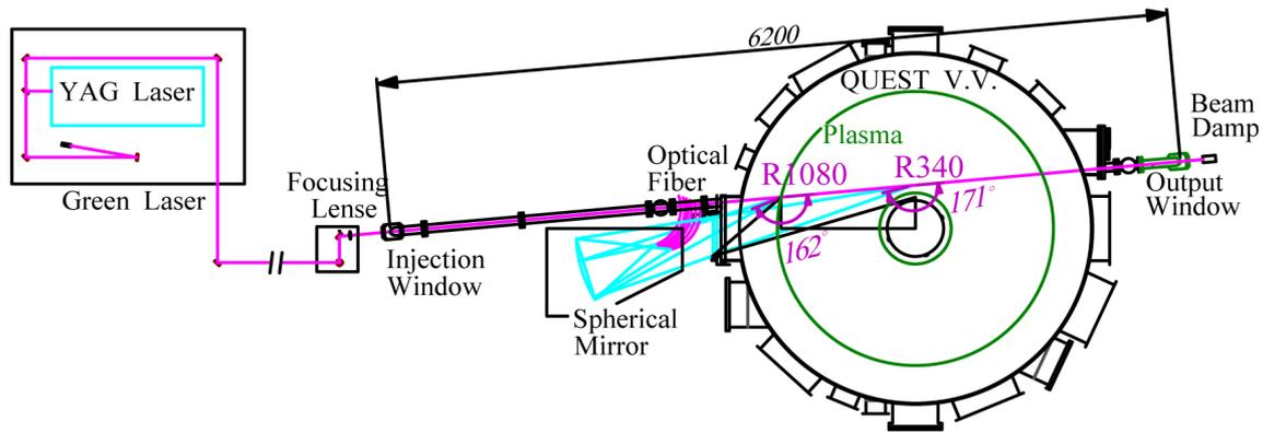
Fig. 1 Arrangement of the QUEST device and the TS system.
