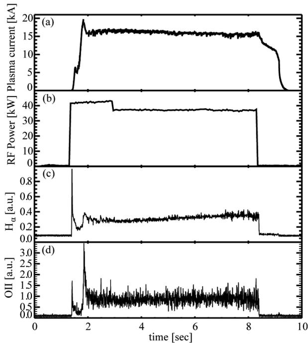
Fig. 4 Time evolution of (a) plasma current, (b) net RF power, (c) H $\alpha$  emission, and (d) OII emission (Shot No.19102).
