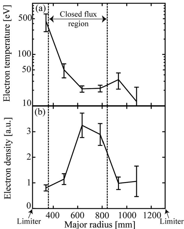
Fig. 7 (a) Electron temperature profile and (b) electron density profile for the inboard null configuration plasma. The dashed lines show the last closed flux surface calculated by RTFIT.
