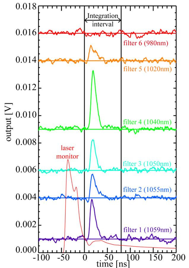
Fig. 5 Averaged scattering signals from 33rd to 82nd laser injections (at 3.3–8.2 s) and three discharges.
