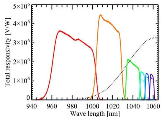
Fig. 3 Spectral sensitivity of each wavelength channel of the polychromator. The black dotted curve shows a Maxwell distribution of 80 eV.
