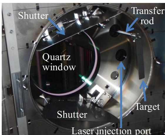
Fig. 2 Vacuum-side photograph of the laser injection and correcting window port (MH14).
