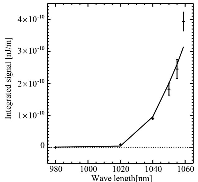
Fig. 6 Fitting to a Maxwell distribution function. The cross points with error bars show the integrated scattering signal. The polygonal line shows fitted values ( $21 \pm 4$  eV).
