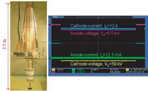
Fig. 2 Photo of 5 GHz prototype klystron and the test results on matched load obtained at the NFRI test bed facility, illustrated by (oscilloscope screen) shot of the cathode (beam) and the anode voltages and current for 304 kW/800 s pulse.
