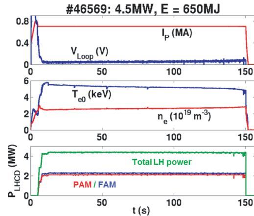
Fig. 8 Tore Supra discharge lasting 150 s, using both the PAM and FAM antennas ( $I_p = 0.7$  MA and line averaged density  $2.5 \times 10^{19} \text{ m}^{-3}$ ).
