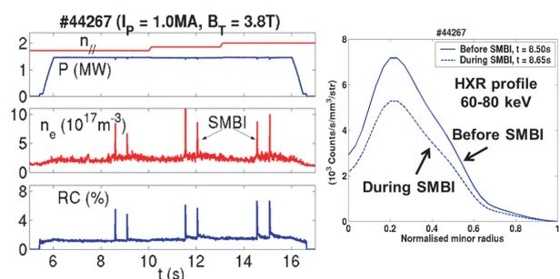
Fig. 6 Left: Time evolution of a discharge with SMBI during LHCD ( $n_{\parallel}$ : parallel refractive index of the waves;  $P$ : coupled LH power ( $P$ );  $n_e$ : density in front of the antenna; RC: reflection coefficient). Right: Radial profile of Hard X-ray 60 keV - 80 keV.
