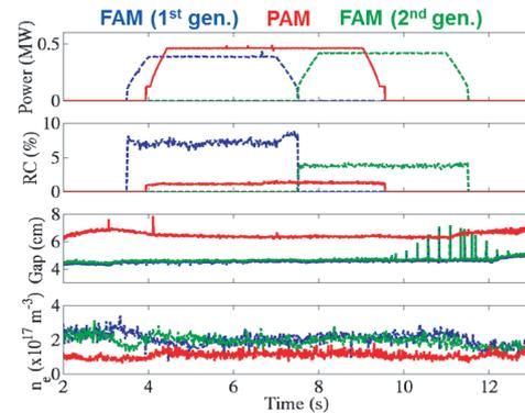
Fig. 5 Comparison of coupling capability between PAM and FAM antennas: time evolution of injected power, reflection coefficient, gap between the plasma and the antenna (red: PAM; blue/green: first and second FAM generations respectively).
