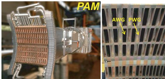
Fig. 4 Left: the Tore Supra LHCD Passive Active Multi-junction launcher. Right: zoom of the front face, showing active waveguides (AWG) alternately with passive waveguides (PWG).
