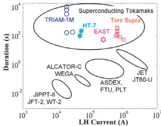
Fig. 1 Progress on LHCD experiments in tokamaks: plasma duration versus LH driven current (ALCATOR-C [22], ASDEX [23], FTU [24], JET [25], JT60 [26], JT60-U [27], PLT [28], WEGA [29]).
