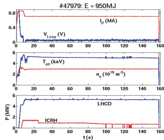
Fig. 9 Combined LHCD&ICRH Giga-Joule discharge with a non-inductive current fraction of 80% (plasma current 0.7 MA, line averaged density  $\sim 3 \times 10^{19} \text{ m}^{-3}$ ). At  $t \sim 80$  s, the ICRH power is decreased by real time protection control because an overheating of Langmuir probes was detected.
