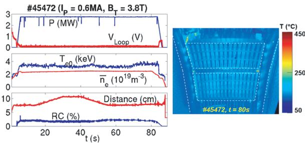
Fig. 7 Demonstration of ITER-relevant capability of the PAM launcher. Left: 25 MW/m<sup>2</sup> over 78 s and good coupling at long plasma-antenna distance (RC < 2%); right: efficient cooling temperature of the antenna front face < 250°C (hot spots correspond to a thermocouple wire and Langmuir probes).
