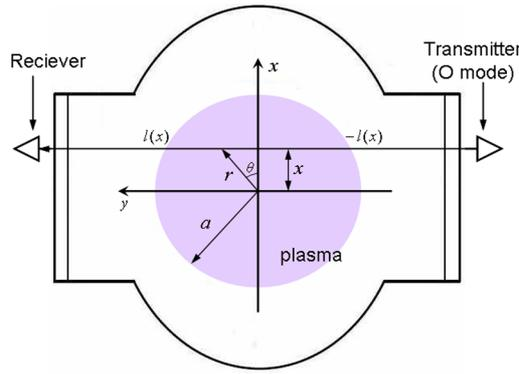
Fig. 2 Schematic view of GAMMA 10 cross section in the plug cell.
