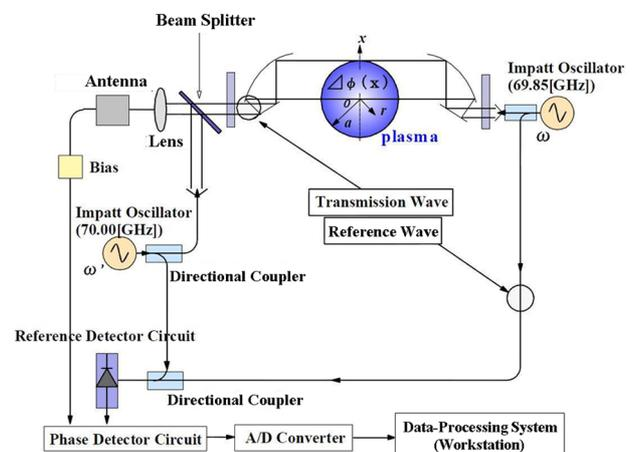
Fig. 1 Schematic diagram of phase-imaging device.
