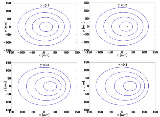
Fig. 3 Asymmetric plasma contour distribution in terms of  $\gamma$ , which is used in the FDTD method.
