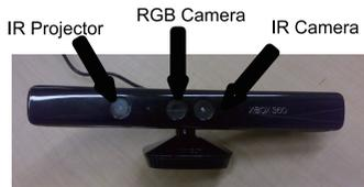
Fig. 4 Microsoft Kinect sensor.
