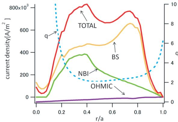
Fig. 3 The red, yellow, green and blue lines are total, boot strap, NBI and ohmic current profile, and light blue dashed line is  $q$  profile.
