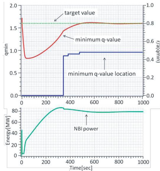
Fig. 4 The red blue and green solid line are minimum  $q$ -value,  $r/a$  where  $q$ -value is minimum and NBI power respectively. The green dashed line is target minimum  $q$ -value.
