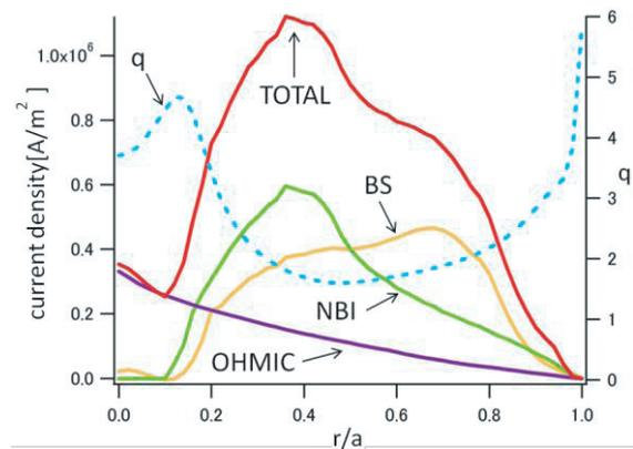
Fig. 5 The red, yellow, green and blue solid lines are total, boot strap, NBI and ohmic current profile, and light blue dashed line is  $q$  profile.
