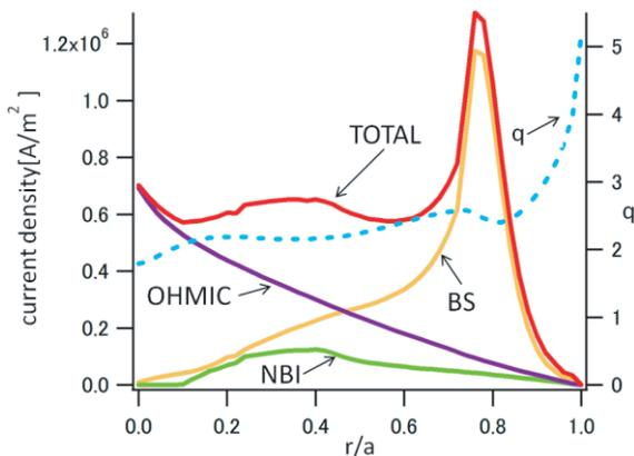
Fig. 7 The red, yellow, green and blue solid lines are total, boot strap, NBI and ohmic current profile, and light blue dashed line is  $q$  profile.
