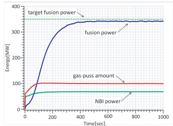
Fig. 1 The blue, red and green solid lines are fusion power, gas-puff amount and NBI power respectively, and green dashed line is target fusion power.
