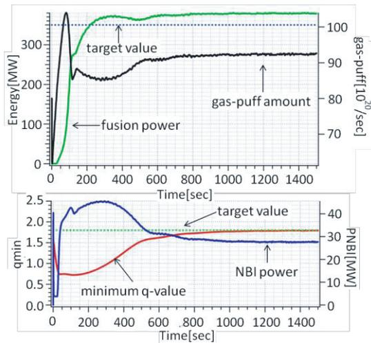
Fig. 6 The green, black, blue and red solid lines are fusion power, gas-puff amount, NBI power and minimum  $q$ -value respectively, and blue and green dashed lines are target fusion power and target minimum  $q$ -value respectively.
