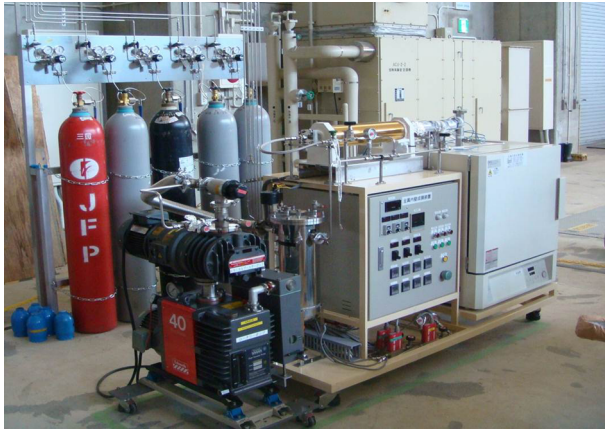
Fig. 1 Large area MOCVD apparatus in NIFS.
