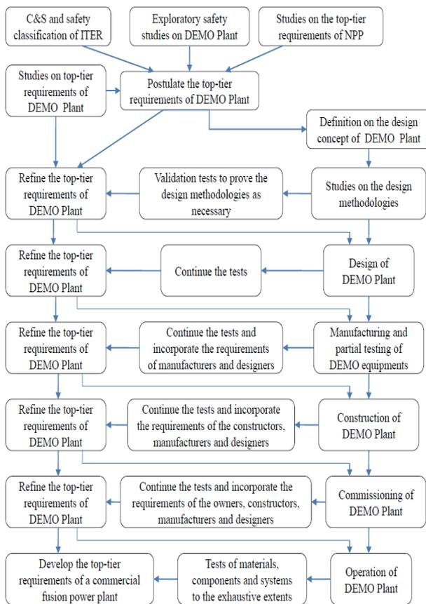
Fig. 2 Proposed Design Processes for K-DEMO1.
