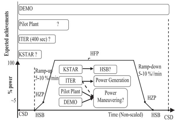
Fig. 1 Expected achievement of the experimental devices.
