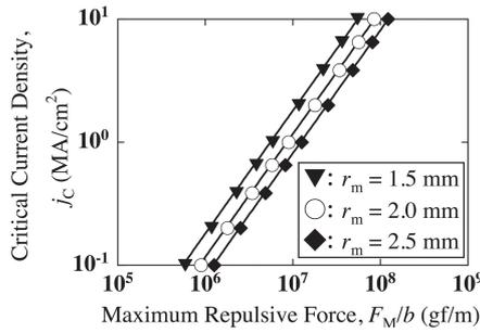
Fig. 1 Dependence of the critical current density  $j_C$  on the maximum repulsive force  $F_M$ .
