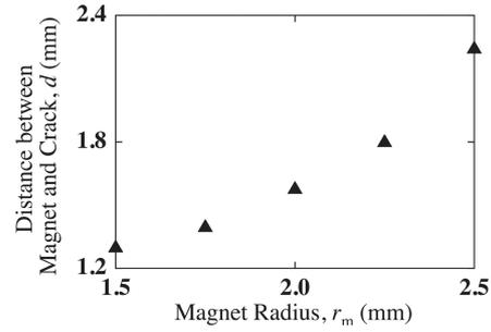
Fig. 3 Dependence of the distance  $d$  on the radius  $r_m$  for  $j_C = 4$  MA/cm<sup>2</sup> and  $L_c = 12$  mm.
