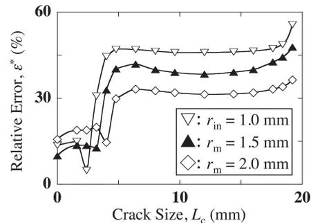
Fig. 6 Dependence of the relative error  $\varepsilon^*$  on the crack size  $L_c$ .
