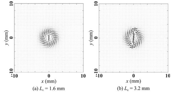
Fig. 5 The spatial distribution of the shielding current density for  $I_0 = 60$  mA and  $r_{in} = 1$  mm at time  $ft = 1.2$ . Here, the thick line indicates the crack.
