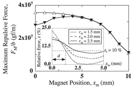
Fig. 2 Dependence of the maximum repulsive force  $F_M$  on the magnet position  $x_m$  for  $r_m = 2$  mm,  $j_C = 4$  MA/cm<sup>2</sup>. Here, the symbols,  $\Delta$  and  $\nabla$ , show  $L_c = 0$  mm and  $L_c = 12$  mm, respectively. The inset indicates the dependence of the relative error  $\varepsilon$  on  $x_m$  for  $r_m = 2$  mm,  $j_C = 4$  MA/cm<sup>2</sup> and  $L_c = 12$  mm.
