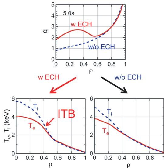
Fig. 6 Comparison of the  $q$  profile at 5 s with and without ECRF during the  $I_p$  ramp-up (top figure). Difference in the  $T_e$  and  $T_i$  profiles with 8 MW of NB injection into these target  $q$  profiles.
