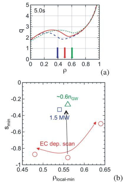
Fig. 5 (a) Change in the  $q$  profile when the ECRF deposition (3 MW) was scanned as illustrated with arrows. (b) A plot of  $s_{\min}$  and  $\rho_{\text{local-min}}$ . Circles: for the cases shown in (a). Square: when the ECRF power was halved to 1.5 MW. Triangle: when  $n_{e0}$  is doubled.
