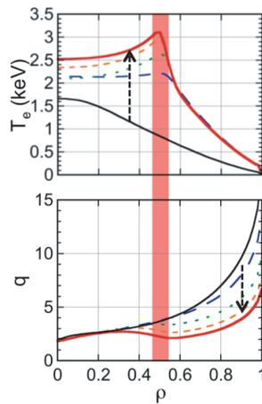
Fig. 4 Temporal evolution of the  $T_e$  and the  $q$  profiles at 1.5 s (thin solid line), 2 s (broken line), 3 s (dotted line), 4 s (dashed line) and 5 s (bold solid line). The arrow in each boxes indicates direction of the evolution from 1.5 s to 5 s. Hatched region at  $\rho \sim 0.5$  indicates the ECRF power deposition.
