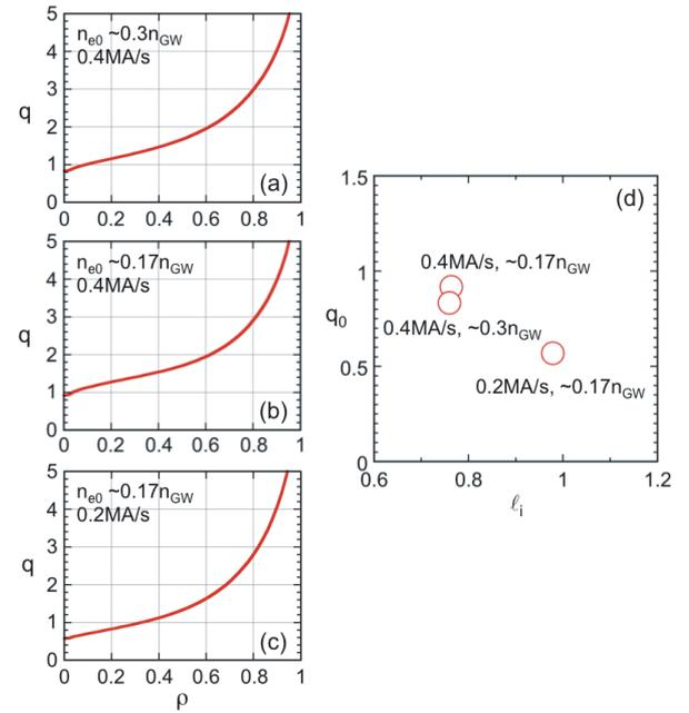
Fig. 2 (a)~(c), the  $q$  profile at 5 s for various combination of  $n_{e0}$  and  $dI_p/dt$ . Plot of  $q_0$  against  $l_i$  corresponding to (a)~(c).
