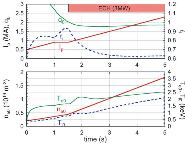
Fig. 3 The temporal evolution of  $I_p$ ,  $l_i$ ,  $q_0$ ,  $n_{e0}$ ,  $T_{e0}$  and  $T_{i0}$  in a 2.3 MA/1.7 T plasma with 3 MW of ECRF.
