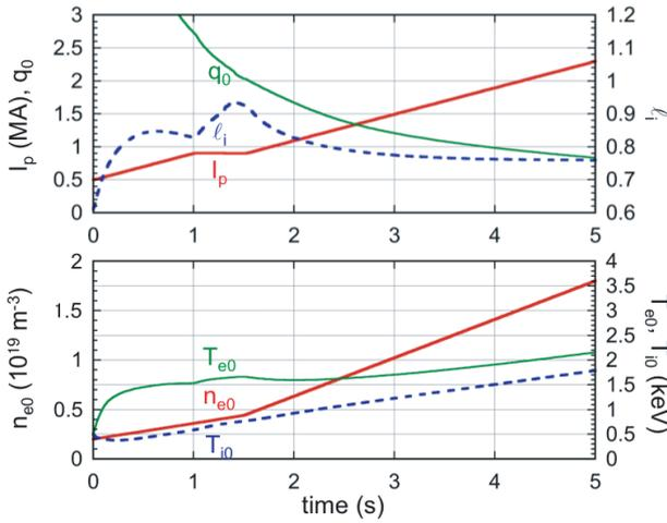
Fig. 1 The temporal evolution of  $I_p$ ,  $l_i$ ,  $q_0$ ,  $n_{e0}$ ,  $T_{e0}$  and  $T_{i0}$  in a 2.3 MA/1.7 T Ohmic plasma.
