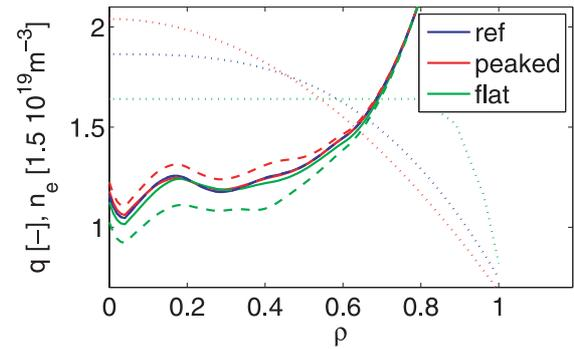
Fig. 5 Effect of flat or extra peaked  $n_e$  profile. Plotted are  $n_e$  and  $q$  profiles at 80 s for the 3 cases (see legend), without (dashed lines) and with adapted heating scheme (full lines).
