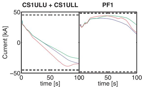
Fig. 4 Some of the coil currents as calculated by FREEBIE. Shown are the currents in the two most critical coils: the central solenoid coils CS1ULU+CS1ULL, and the poloidal field coil PF1, for a typical heating scheme (full red lines) and for a case with only ohmic heating (dashed red lines). The maximum and minimum allowed currents are plotted in black.
