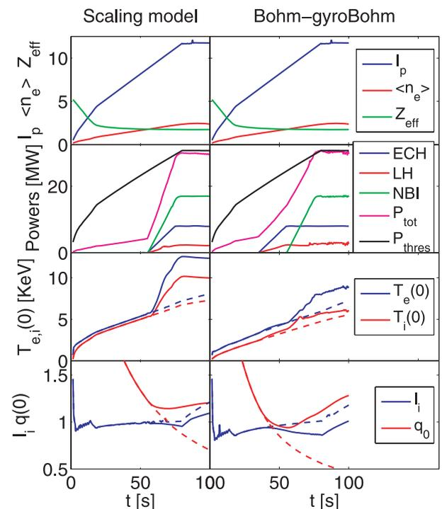
Fig. 2 Time traces of the optimized scenario for the reference case, assuming scaling model (left panels) or Bohm-gyroBohm model (right panels). For comparison the figure also shows the time traces of  $T_{e,i}(0)$ ,  $I_i$  and  $q(0)$  without any additional heating (dashed lines).
