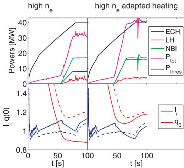
Fig. 6 Time traces of powers,  $q(0)$  and  $I_i$  for the high  $n_e$  case with the heating scheme of the reference scenario (left) and with adapted heating scheme (right). For comparison the lower panels also show the time traces of  $q(0)$  and  $I_i$  of the reference scenario (dashed lines). Without modified heating scheme,  $q(0)$  drops far below 1 and  $I_i$  rises too high (i.e. above 1); these unwanted features are avoided with the adapted heating scheme.
