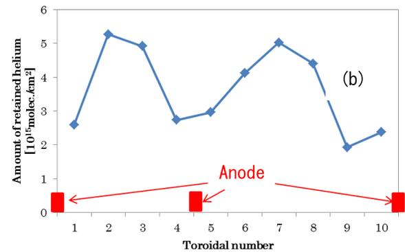
Fig. 7 Toroidal distribution of (a) hydrogen and (b) helium.
