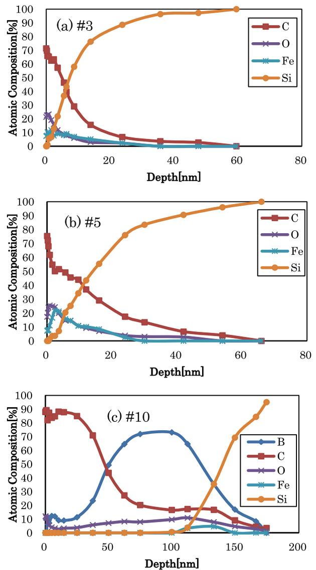
Fig. 3 Depth profile of atomic composition for (a) #3, (b) #5 and (c) #10 probe.
