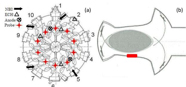
Fig. 1 Locations of the material probes. (a) is upper view and (b) cross sectional view for the LHD.
