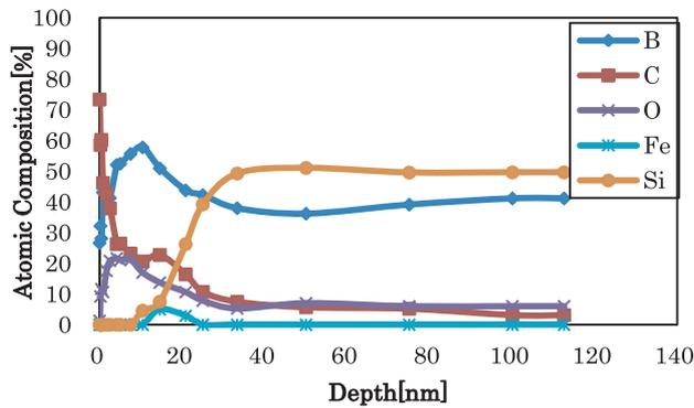
Fig. 5 Depth profile of atomic composition for #1 probe.
