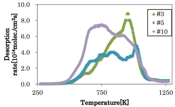
Fig. 2 Thermal desorption spectra of H<sub>2</sub> for #3, #5 and #10.
