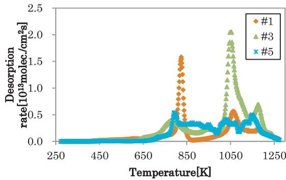
Fig. 4 Thermal desorption spectra of helium for #1, #3 and #5.
