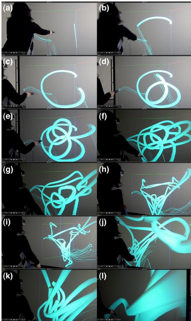
Fig. 6 Visualization of an ABC-flow with the VR timeline method in CAVE. (a) to (e) show 3-D drawing phase of the initial curve. (f) to (l) are snapshot sequence of the time development of the frozen-in field line or the timeline.
