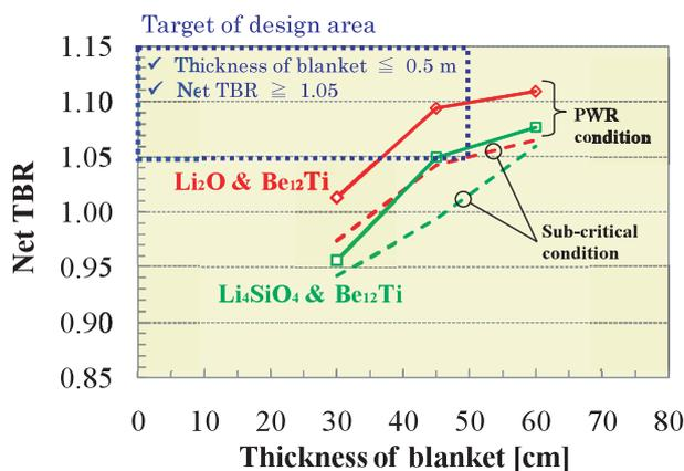
Fig. 9 Dependence of net TBR on blanket in thickness.
