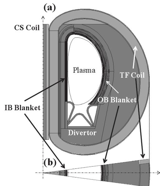
Fig. 7 MCNP calculation model for SlimCS (a: vertical cross section in the 3-D model and b: horizontal cross section at mid-plane).
