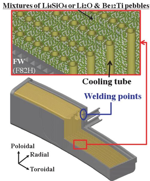
Fig. 2 Interior design of blanket by PWR coolant condition.
