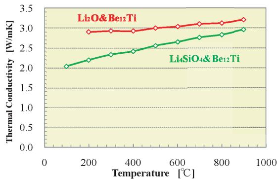
Fig. 5 Thermal conductivities of breeder and multiplier.
