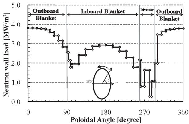
Fig. 8 Distribution of neutron wall load for SlimCS.
