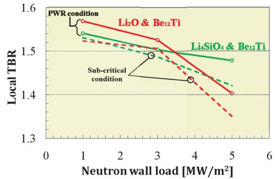
Fig. 6 Dependence of local TBR on neutron wall load.
