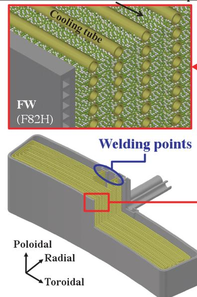
Fig. 1 Interior design of blanket by sub-critical water condition.
