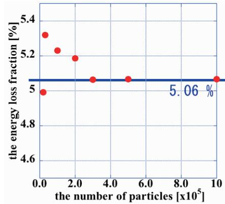
Fig. 5 The energy loss fractions of  $\alpha$  particle  $\eta_{\text{loss}}$  are calculated until  $\alpha$  particles are thermalized for  $N_\alpha = 1000 \sim 100,000$ .
