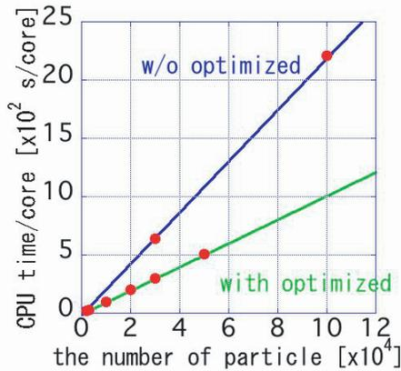
Fig. 6 The calculation time for each case. The calculation time increases linearly with the number of test particles. On the blue line, the calculations have not been optimized. On the green line, the calculations have been optimized.
