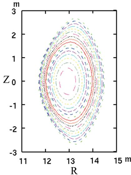
Fig. 1 The flux contour for the NC configuration in the real coordinate.  $R$  is the major radius and  $Z$  is the minor radius in vertical direction.
