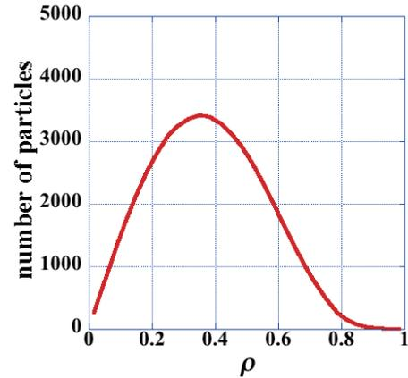
Fig. 2 The initial radial profile of  $\alpha$  particles, for  $n(0) = 2.0 \times 10^{20} \text{m}^{-3}$ , with 50,000 test particles.
