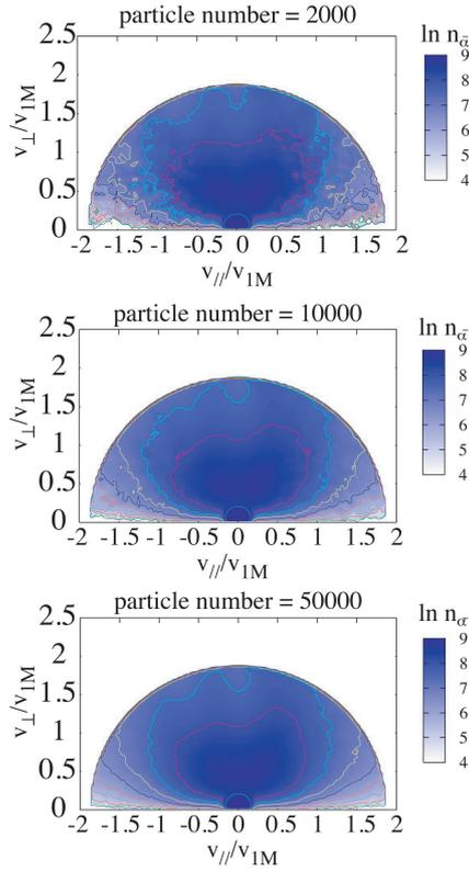
Fig. 3 Contour plots of the particle density in velocity space for the cases  $N_\alpha = 2000$ , 10,000, and 50,000. The contour levels are spaced logarithmically in the velocity space distribution.
