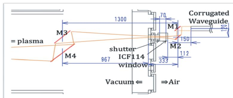
Fig. 1 Schematic layout plan of the ECE antenna system in the outer port of the torus in the LHD. The antenna consists of four mirrors, namely, M1, M2, M3, and M4 in the increasing order of distance from the waveguide in air. The layout is determined by the spot size at the plasma and the beam is passed through the tube between M2 and M3, matching it to the corrugated waveguide.
