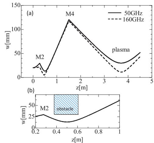
Fig. 2 (a) Beam size evolution at 50 GHz and 160 GHz. (b) Enlarged view around the waist position in a narrow tube. Stainless steel pipe 30 mm in radius is depicted as an obstacle.
