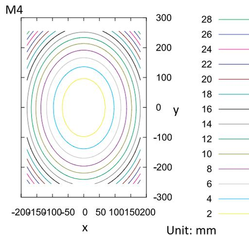
Fig. 4 Constant-phase mirror surface of M4. The value of contour lines is the height from the bottom at the center.
