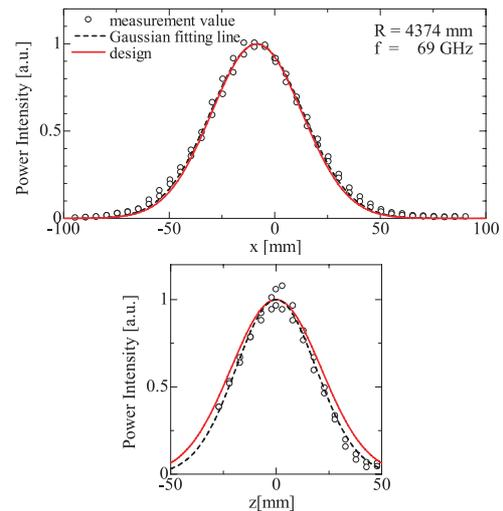
Fig. 5 Comparison between the measured power profile and the Gaussian beam profile. Intensity is normalized by the maximum of a fixed line of a measured value.
