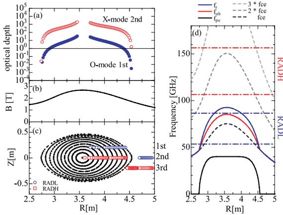
Fig. 6 (a) Optical depth profile. (b) Magnetic field profile along the ECE sight line. (c) Locations of the measurement points on the heterodyne radiometer channel. Sight line is on the midplane. Fundamental and third harmonic resonance points are drawn on the upper and lower lines to facilitate visualization. (d) Characteristic frequency profiles  $f_r$ : right hand cutoff frequency;  $f_{uh}$ : upper hybrid resonance frequency;  $f_{pe}$ : plasma frequency.
