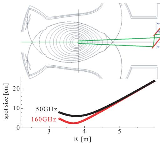
Fig. 3 Spot size at 50 GHz and 160 GHz in the plasma area. Waist position is set around the magnetic axis.
