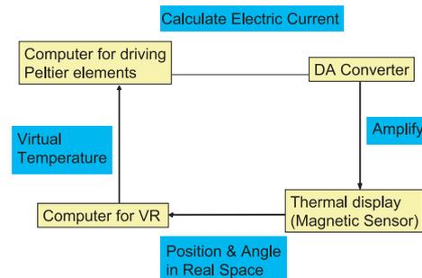
Fig. 3 Data flow between the real thermal sense and the virtual thermal data.
