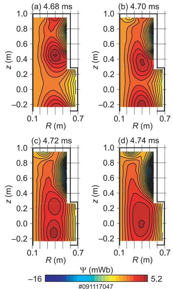
Fig. 4 Time evolution of poloidal magnetic flux contours during the PF + CS discharge at (a) 4.68 ms, (b) 4.70 ms, (c) 4.72 ms, and (d) 4.74 ms. Reconnection of the magnetic surface is clearly observed by poloidal magnetic flux measurement.
