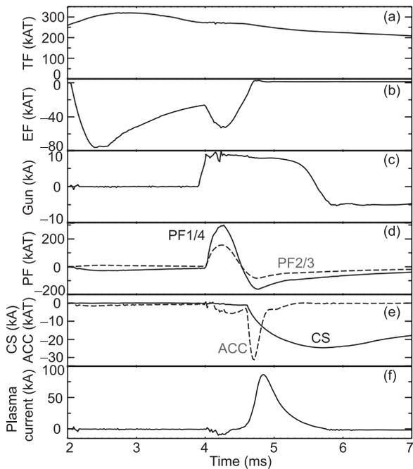
Fig. 3 Typical discharge of UTST plasma by DNM assisted by the CS coil. Time evolutions of the currents of the (a) TF coil, (b) EF coils, (c) washer guns, (d) PF coils, (e) CS coil/ACC coils, and (f) plasma. Positive direction is counterclockwise.
