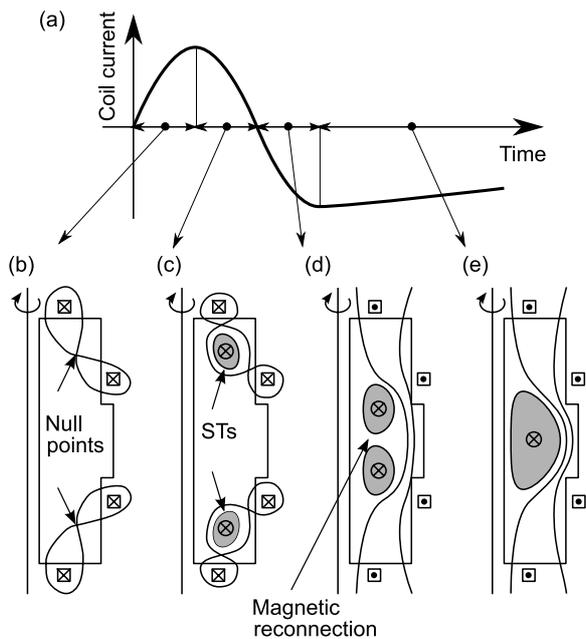
Fig. 1 Drawings illustrating DNM as used in the UTST. (a) Current of the PF coils used for DNM. (b) Outer PF coils generate two null points inside the vacuum vessel. (c) Two STs are generated at the null points. (d) When the PF coil current is reversed, the STs are pushed toward the midplane. (e) STs merge to form a single high-beta ST.
