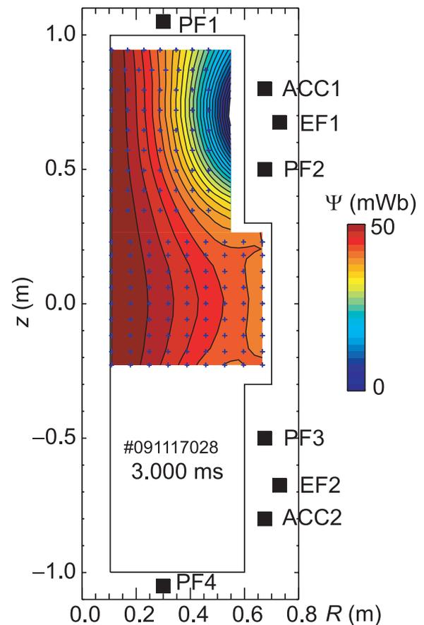
Fig. 2 Schematic of the UTST plasma merging device. Locations of EF1 and 2, PF1–4, and ACC1 and 2 coils are illustrated. Crosses indicate the positions of the  $B_z$  and  $B_t$  pickup coils. Plot shows the contours of the poloidal magnetic flux generated by the EF coils.
