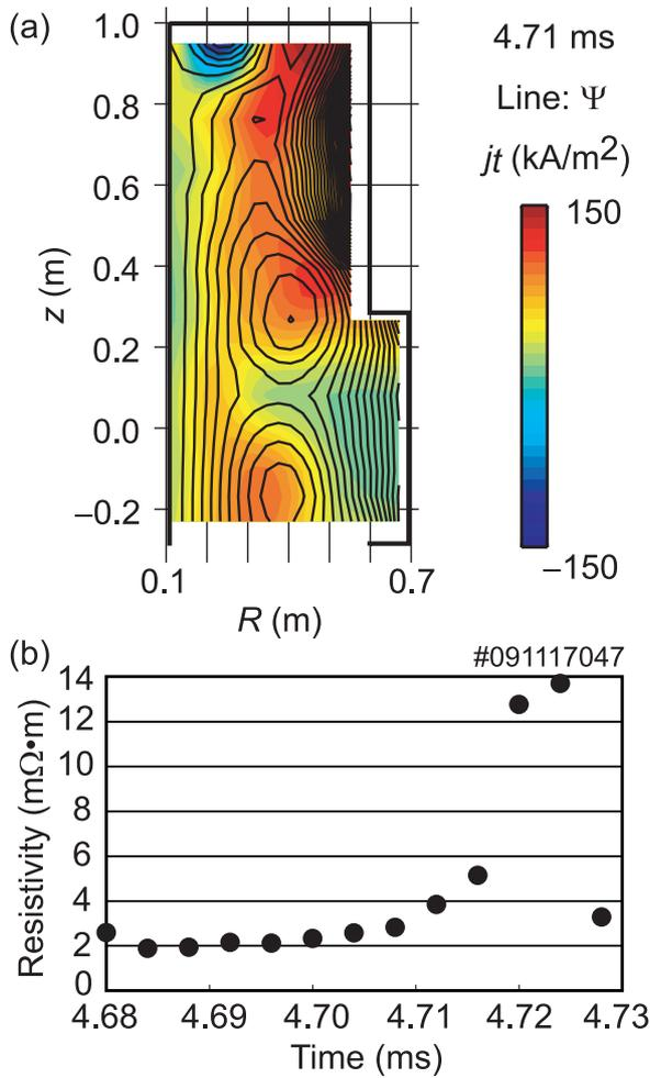
Fig. 5 (a) Poloidal magnetic flux contours with toroidal current density (by color) during PF + CS discharge at 4.71 ms. (b) Time evolution of the effective resistivity at the current sheet.
