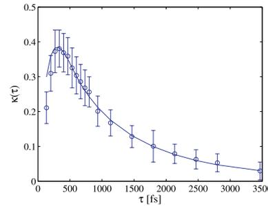
Fig. 2 Measured (open circles) and calculated (solid line) relative absorption as a function of the delay between the pump and the probe.
