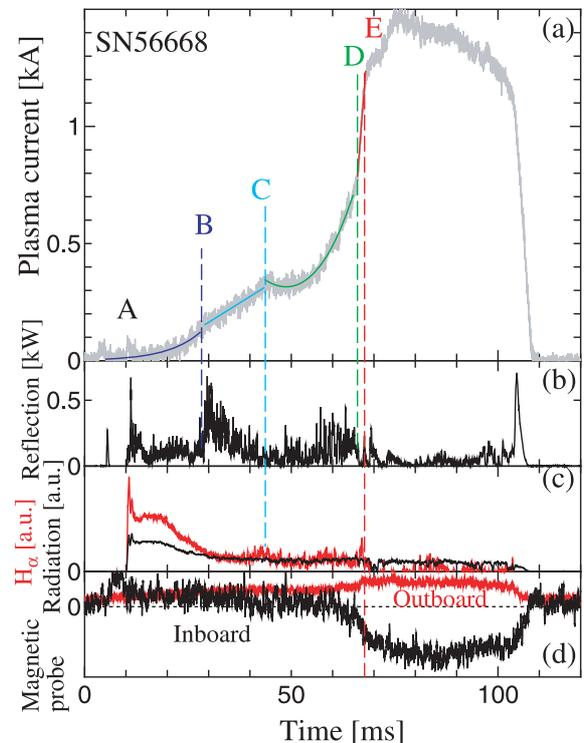
Fig. 4 Current jump with a strong vertical field. Current jump is divided into four phases on the basis of the plasma current waveform (a). ECH reflection power (b), hydrogen emission and radiation (c), and outboard and inboard vertical fields (d) are also plotted.
