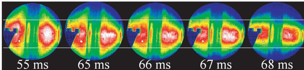
Fig. 5 Visible camera images during a current jump. Image at 55 ms is a sample before the vertical shrinkage. At 66 ms, the ECH reflection signal is attenuated. The vertical field at the outboard signal reaches maximum value at 67 ms.
