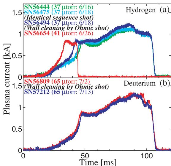
Fig. 1 Waveforms of plasma current after the start of vacuum pumping. (a) ECH start-up discharges before and after about 100 Ohmic discharges. (b) Similar sequence, but the effect of the Ohmic discharges is negligible.
