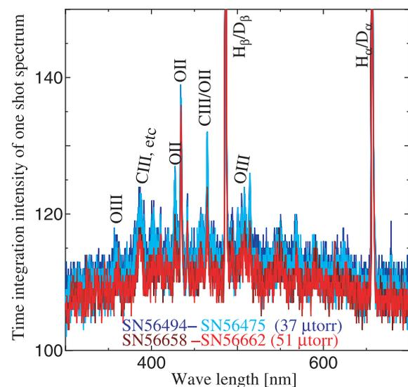
Fig. 2 Spectra of time-integrated visible emission. Before the Ohmic discharge, the oldest shot emission (sky blue) is weaker than that in newer shots (blue). Emissions after the Ohmic discharge (red) are identical and are weaker than those before cleaning. Note that the filling hydrogen pressure was higher after cleaning.
