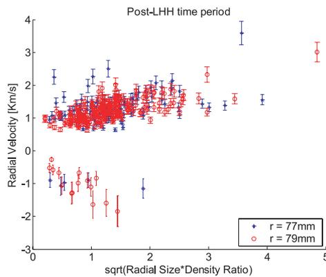
Fig. 4 Radial velocity versus the square root of the product of radial size with density ratio, for blobs found after heating, at 2 radial positions.
