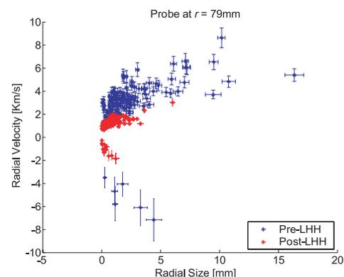
Fig. 3 Radial velocity and radial size estimates for blobs detected in periods before and after LHH, at the HFS and  $r = 79$  mm.
