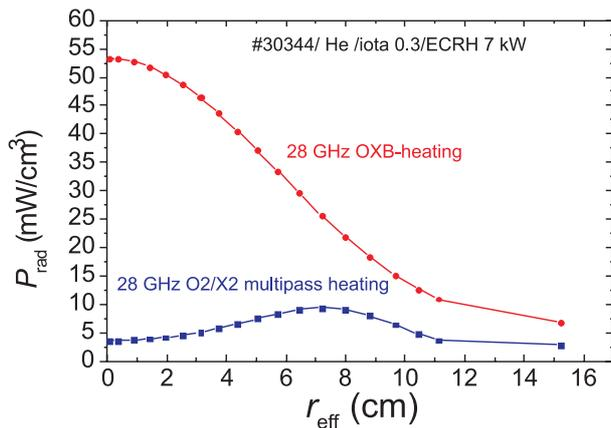
Fig. 3 Reconstructed radiation profiles measured with the bolometer camera before (blue) and during (red) OXB mode heating phase.
