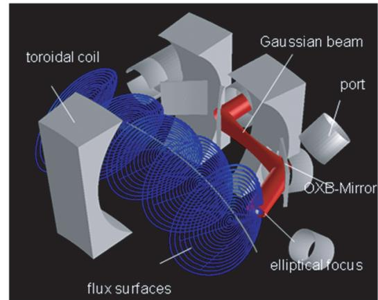
Fig. 1 Setup of the focusing mirror system inside the plasma vessel. The beam trajectory is indicated in red, the magnetic flux surfaces in blue.
