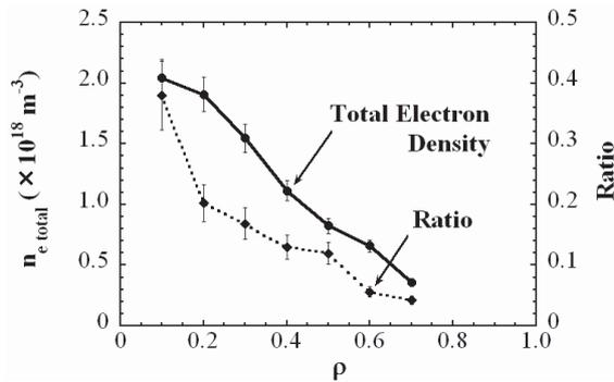
Fig. 5 Radial profiles of total electron density (solid line) and ratio of suprathermal electrons to total electron density (dashed line), respectively.
