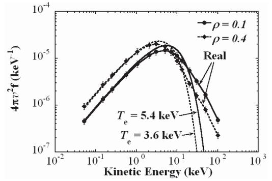
Fig. 7 Real and maxwellian energy-distribution functions for the low-density ECH plasmas. Real distribution is obtained from experimental x-ray energy spectra. For the bulk maxwellians,  $T_e(0)$  is 5.4 and 3.6 keV at  $\rho = 0.1$  and 0.4, respectively.
