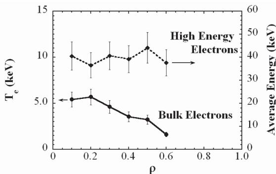
Fig. 6 Radial profiles of bulk electron temperature (solid line) and average energy of suprathermal electrons (dotted line).
