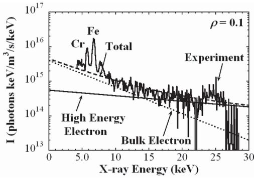
Fig. 4 Abel inverted x-ray energy spectra obtained from the experimental and calculated results. X-ray energy spectra calculated for the bulk component (dotted line) and the high energy component (solid line) are plotted with the total spectrum of two components (dashed line).
