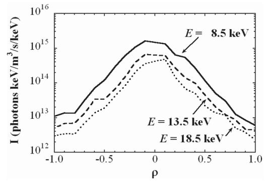
Fig. 3 Radial profiles of Abel inverted x-ray spectra at energies of 8.5, 13.5 and 18.5 keV.
