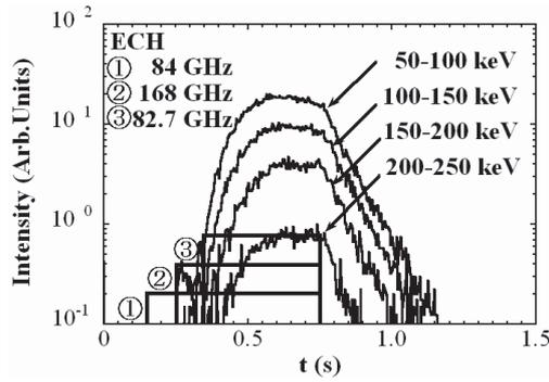
Fig. 1 Time evolution of the hard x-ray emissions measured with the germanium-semiconductor detector. The heating duration of ECH is also illustrated.
