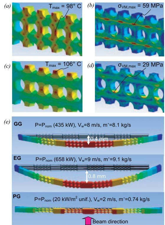
Fig. 5 Thermo-structural analyses performed with the ANSYS code on the reference scenario: (a) and (b) Temperature and Von Mises equivalent stress on the EG; (c) and (d) Temperature and Von Mises equivalent stress on the GG; (e) Out of plane deformations of the three grids.
