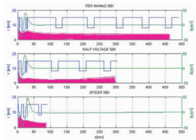
Fig. 1 Ion beam trajectories simulated with SLACCAD. Also the aperture profiles and the magnetic field by suppression magnets is sketched.
