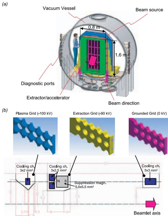
Fig. 2 Scheme of the grids for the 100 kV accelerator: (a) Design overview; (b) Detailed view of the grids.
