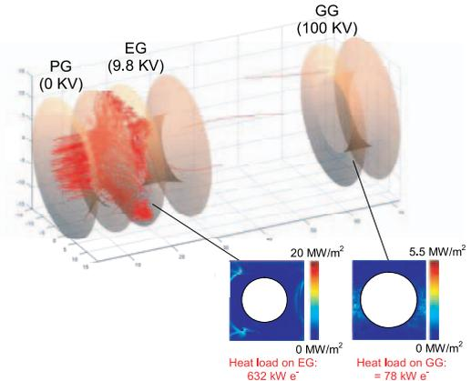
Fig. 4 EAMCC simulation of the beam in the 100 kV accelerator: the particle trajectories and stripping reaction are simulated with a Monte Carlo approach in a domain with electrical and magnetic fields. The power corresponding to the whole accelerator (1280 beamlets) is reported.
