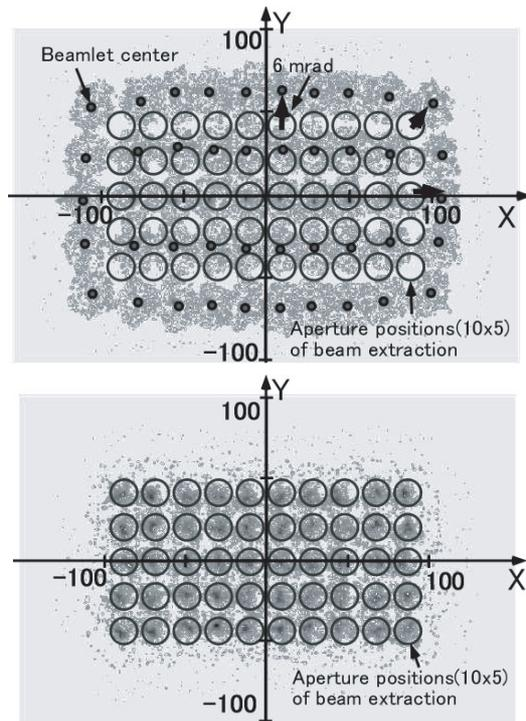
Fig. 6 Calculated beam footprints at 3.5 m downstream from the GRG (a) before and (b) after proper aperture offset in the extractor. The beam parameter is  $110 \text{ A/m}^2$  of  $D^-$  ion beam current density and 340 keV at beam energy. Opened circles represent the original aperture positions.
