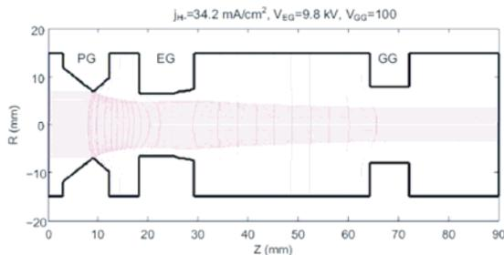
Fig. 3 SLACCAD simulation of the beam optics: equipotential lines (blue) and particle trajectories (magenta) are estimated by integration of the Poisson's equation.
