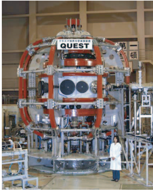
Fig. 2 The vacuum vessel and TF, PF coils of QUEST
