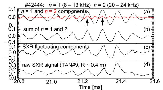
Fig. 2 Time evolution of  $n = 1$  and  $n = 2$  modes on SXR Ch. 9 ( $R_{\text{tan}} = 0.4$  m). (a)  $n = 1$  and  $n = 2$  components of SXR signal [a.u.], (b) sum of the two modes, (c) fluctuating components of the SXR signal [a.u.], (d) raw SXR signal.
