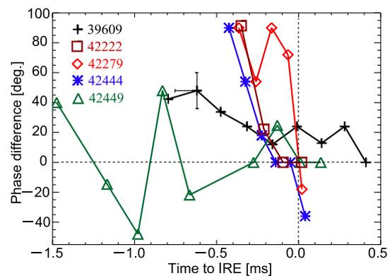
Fig. 3 Time evolutions of the phase difference between the positive peaks of  $n = 1$  and  $n = 2$  modes near the inversion radius extracted from SXR data in several discharges.
