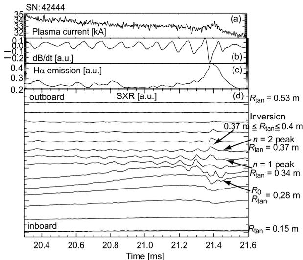
Fig. 1 Waveforms with an IRE. (a)  $I_p$  [kA] (plasma current), (b)  $dB/dt$  [a.u.] from the  $n$ -coil. (c)  $H_{\alpha}$  emission [a.u.] (d) SXR signals obtained by the tangential SXR camera.
