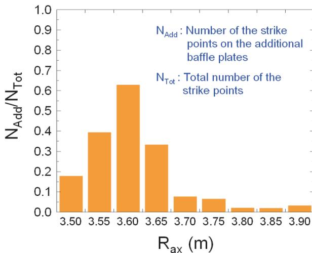
Fig. 5 Ratio of the number of strike points on the additional baffle plates to that of all strike points in various magnetic configurations ( $R_{ax} = 3.50 \sim 3.90$  m).
