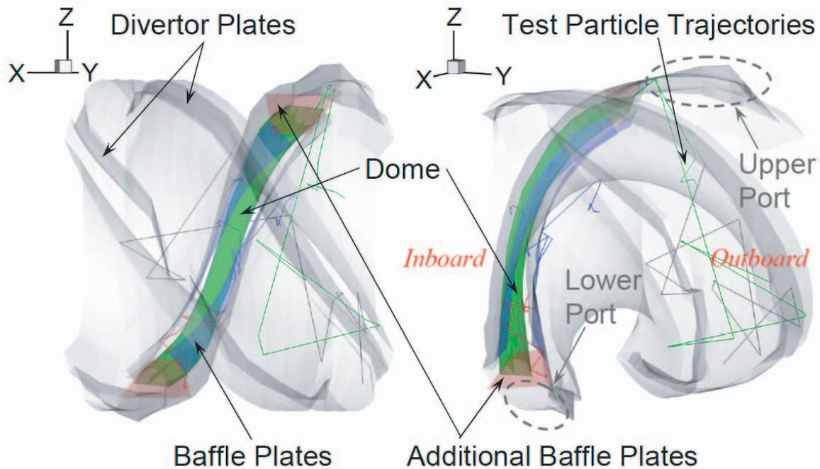
Fig. 2 Three-dimensional model for neutral particle transport simulation in the closed divertor configuration with additional baffle plates (target plates) installed at both toroidal ends of a dome structure in the inboard side of the torus. The closed divertor consists of baffle plates, a dome structure, and slanted divertor plates, which are installed in the inboard side of the torus. Test particle trajectories calculated using neutral particle transport simulation are also shown.
