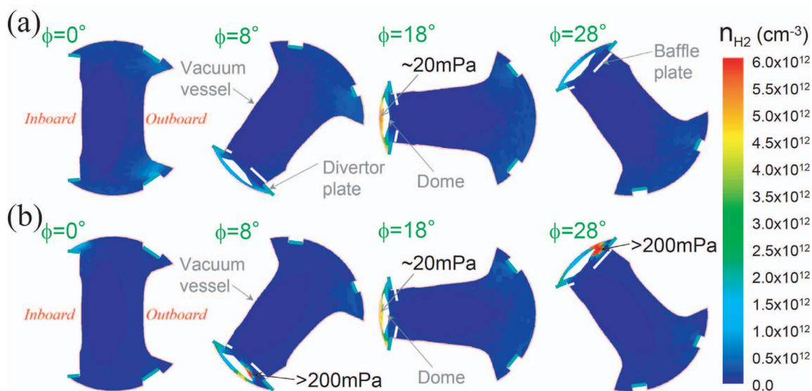
Fig. 6 Four poloidal cross-sections of the calculated density profile of neutral hydrogen molecules for the closed divertor configuration (a) and the configuration with the additional baffle plates ( $R_{\text{ax}} = 3.60 \text{ m}$ ) (b).
