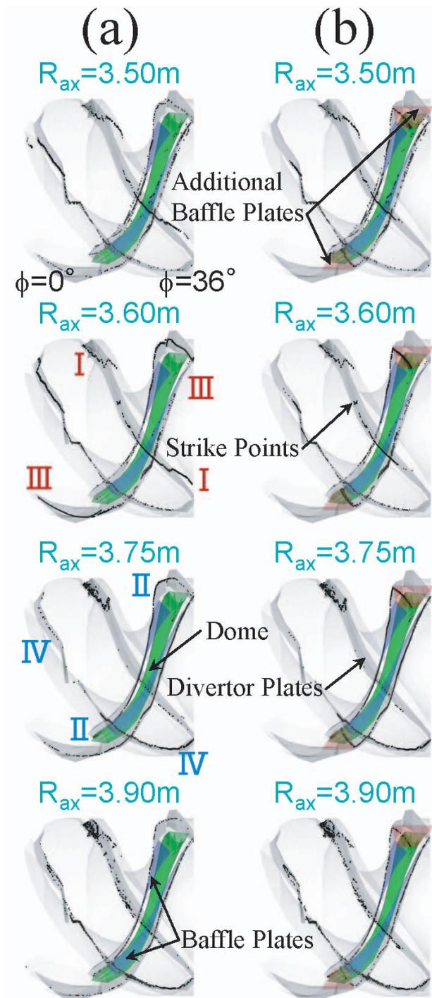
Fig. 3 Toroidal and poloidal distribution of strike points (black dots) in the closed divertor configuration without (a) and with (b) additional baffle plates in various magnetic configurations ( $R_{ax} = 3.50$  m ~  $3.90$  m).
