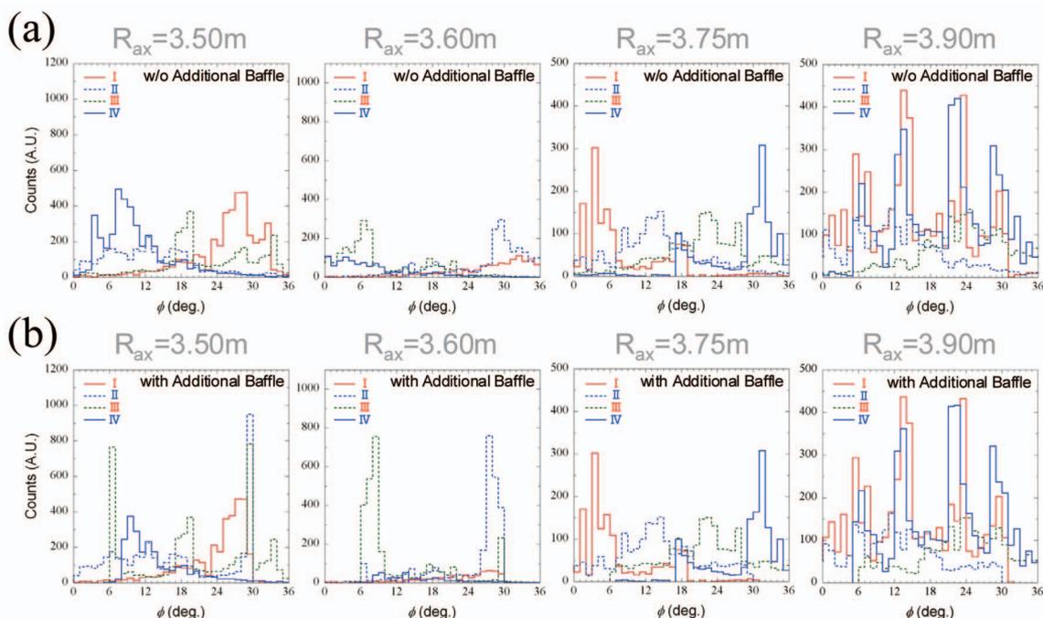
Fig. 4 Histograms of the number of strike points along four divertor legs in the case with (a) and without the additional baffle plates (b) in various magnetic configurations ( $R_{ax} = 3.50 \sim 3.90$  m). The toroidal and poloidal positions of the strike points along the four divertor legs (I, II, III, IV) are indicated in Fig. 3 (a).
