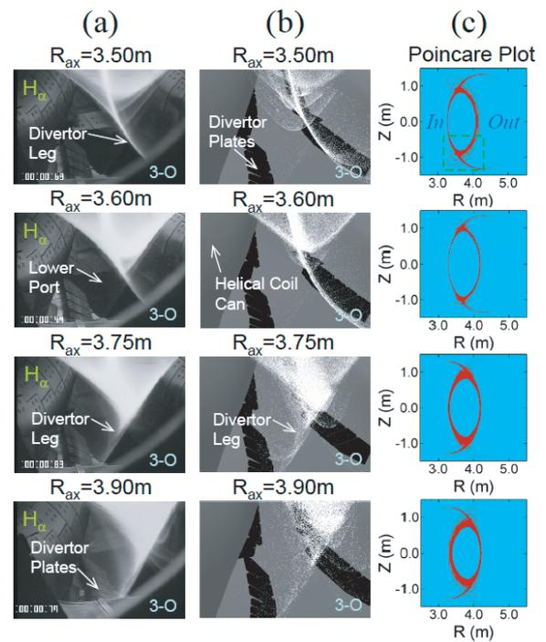
Fig. 1 Images of  $H_\alpha$  emission near a lower port (a) and three-dimensional plots of the magnetic field lines in the plasma periphery (white dots) (b), and Poincare plots at a toroidal angle where the shape of the plasma is vertically elongated (c) in various magnetic configurations ( $R_{ax} = 3.50 \text{ m} \sim 3.90 \text{ m}$ ).
