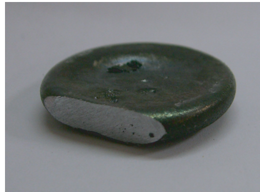
Fig. 4 Pig iron from the 30 GHz mm-waves process.
