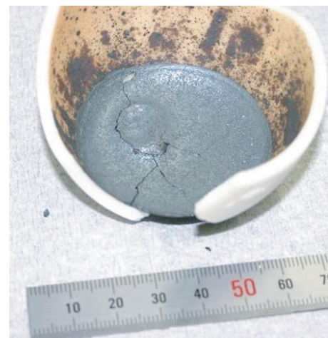
Fig. 6 Sample after 2.45 GHz processing.
