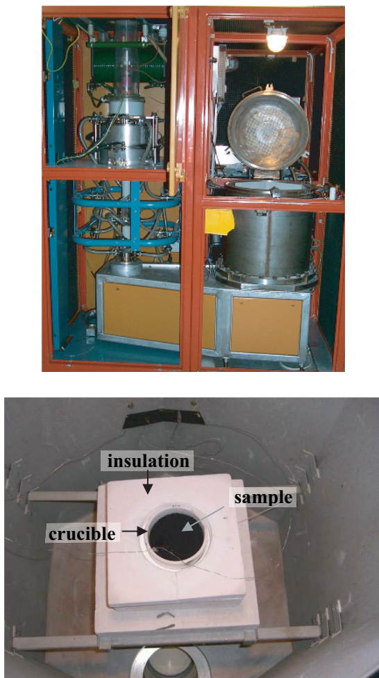
Fig. 1 (a) 30GHz gyrotron system (top), (b) Experimental setup of the mm-wave (bottom).
