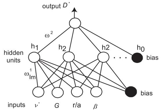
Fig. 4 Schematic view of MLP1 neural network used in calculations of  $D^*$ .
