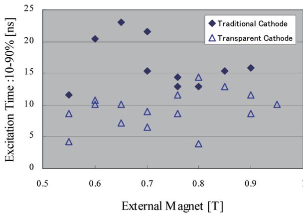
Fig. 6 Excitation time until the first peak: 10% to 90% time. Diamonds represent the excitation time with the traditional cathode. Triangles represent the excitation time with the transparent cathode.
