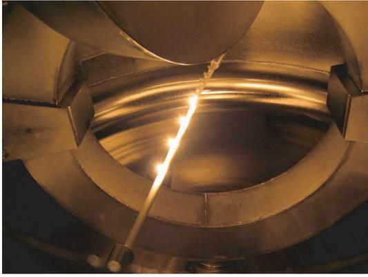
Fig. 2 A picture of the hot emissive filaments mounted on ceramic rods inserted into the magnetic surfaces of CNT.
