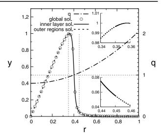
Fig. 1 The radial displacement of the m = 1 internal kink mode for  $2\pi R_0 = 60$  ( $k = 2\pi/R_0$ ). The safety factor q is shown by a dotted-dashed line; the q = 1 surface is located at r = 0.4. The outer and inner layer solutions using the new scheme are indistinguishable from the solution in its full range (0, 1);  $r_{\rm L} = 0.35$ ,  $r_{\rm R} = 0.45$ . Enlargements around the matching points show that each inner layer solution connects smoothly to each outer solution.
