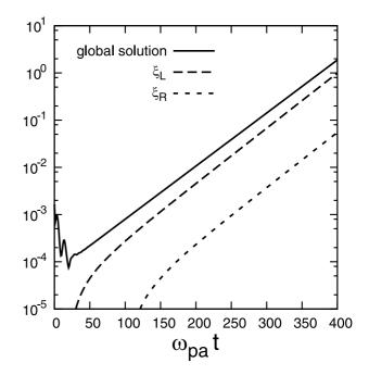
Fig. 2 The evolutions of  $\xi_{\rm R}$  (dotted line),  $\xi_{\rm L}$  (broken line), and the norm of the global solution (solid line). The estimated growth rates of  $\xi_{\rm R}$ ,  $\xi_{\rm L}$  are  $\gamma = 2.7 \times 10^{-2} \omega_{\rm pa}$ , and are close to that from the global solution,  $\gamma = 2.6 \times 10^{-2} \omega_{\rm pa}$  ( $\omega_{\rm pa}$ denotes the Alfven frequency at the plasma surface).
