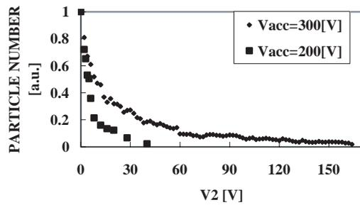
Fig. 6 The total number of electrons hitting the fluorescent screen for  $V_{\text{acc}} = -300 \text{ V}$  and  $V_{\text{acc}} = -200 \text{ V}$ .
