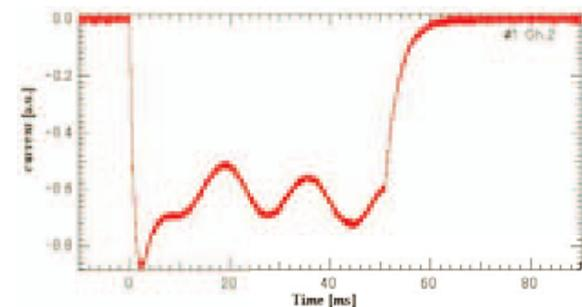
Fig. 5 The time evolution of the current flowing out from the fluorescent screen.
