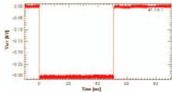
Fig. 4 The time evolution of acceleration voltage applied to the LaB<sub>6</sub> cathode. During the duration time (~50 ms), electrons are emitted from the LaB<sub>6</sub> cathode.
