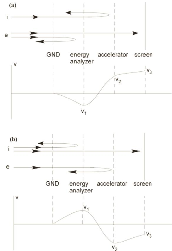
Fig. 1 A schematic drawing of potential distribution along the particle trajectory: (a) for electrons (b) for ions.
