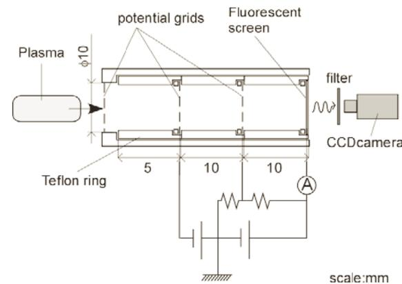
Fig. 2 A schematic drawing of the proposed instrument containing the fluorescent screen and the grided energy analyzer.
