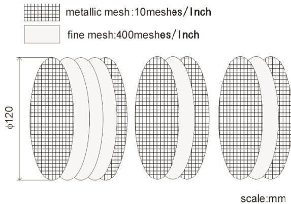
Fig. 3 A schematic drawing of grids; two different sets of grids are used in the grided energy analyzer. All meshes are made of stainless metal (SUS304).
