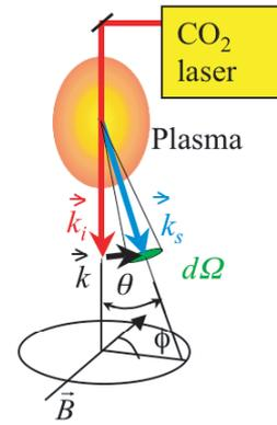
Fig. 5 Schematic diagram of the scattering geometry for the collective Thomson scattering.
