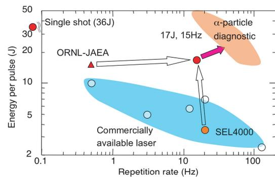
Fig. 1 Progress of the energy and the repetition rate of CO<sub>2</sub> laser for  $\alpha$ -particle diagnostic. Output energy of 17 J at a repetition rate of 15 Hz has been obtained. Maximum output energy of 36 J has been obtained.
