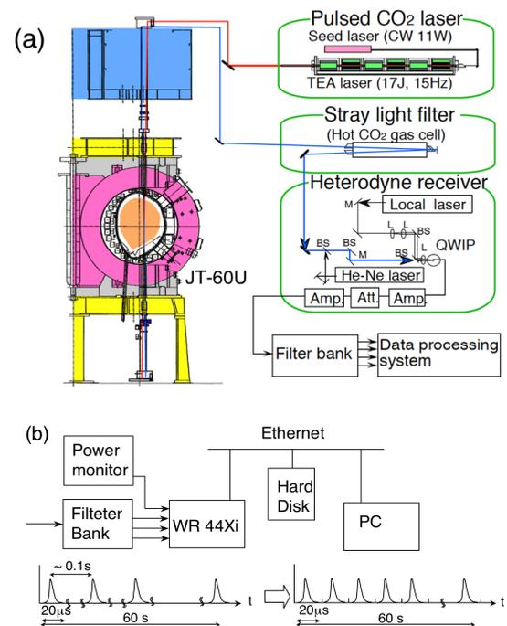
Fig. 3 (a) The CTS system on JT-60U. (b) Data processing system using the digital oscilloscope WaveRunner 44Xi.
