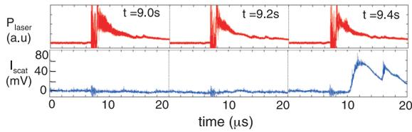
Fig. 4 Waveform of CO<sub>2</sub> laser power monitor,  $P_{laser}$ , and output of the filter-bank (1 ch 0.4 -0.7 GHz),  $I_{scat}$ .
