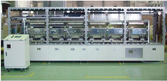
Fig. 2 Newly developed high-repetition CO<sub>2</sub> laser. The size of the casing is 5.3 m long × 1.9 m high × 1.1 m wide.
