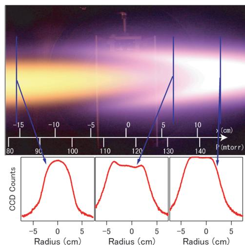
Fig. 1 Typical camera picture of the plasma column streaming from left to right, with the equivalent measured spatial position's dependence on the neutral pressure. Three emission intensity radial profiles at three different points are shown. One can see the recombining front covering the tip of the ionizing plasma.
