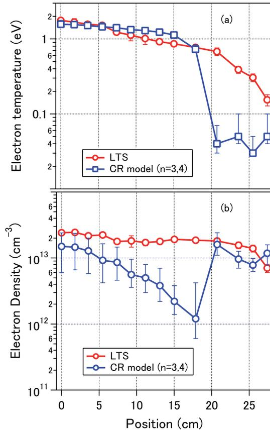
Fig. 2 Comparison of Laser Thomson Scattering and CR model results: (a) Electron temperature profile, (b) Electron density profile.
