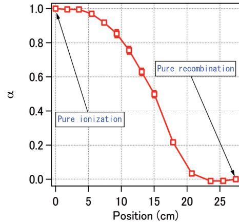
Fig. 3 Profile of the parameter  $\alpha$  as obtained from the fitting of the line intensity ratios according to Eq. (1).
