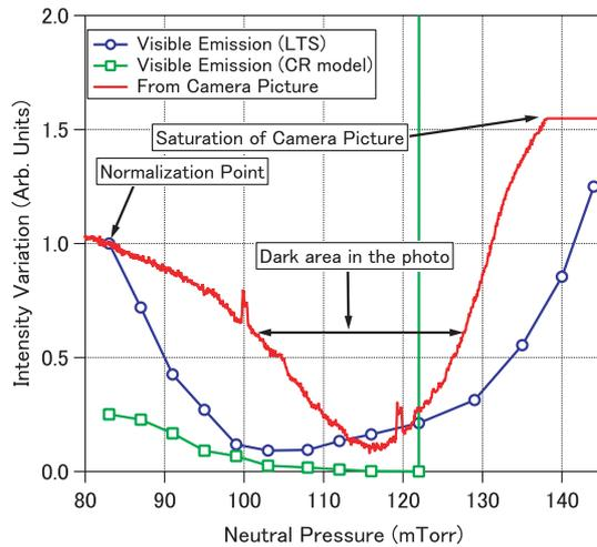
Fig. 4 Relative light emission intensity obtained from camera picture (continuous line), LTS results (circles), CR model results (squares).
