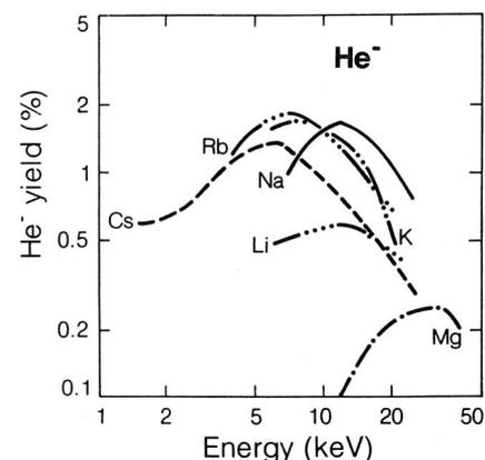
Fig. 1 Charge exchange efficiency of He<sup>+</sup> to He<sup>-</sup> in several alkali metal vapors. The maximum efficiency of lithium is about 0.5 % at the 13 keV of injected He<sup>+</sup> beam [4].
