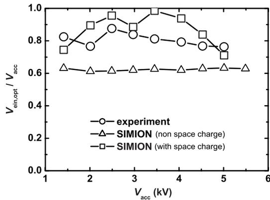
Fig. 3 Einzel lens effect. Ion source gas pressure of  $2-3 \times 10^{-5}$  torr. The optimum einzel lens voltage was 75-87 % of the beam energy at an optimum lens voltage. According to the simulation on SIMION [11], the fraction was about 60 % of the beam energy when the space charge is not considered. The fraction when the space charge is considered shows higher value.
