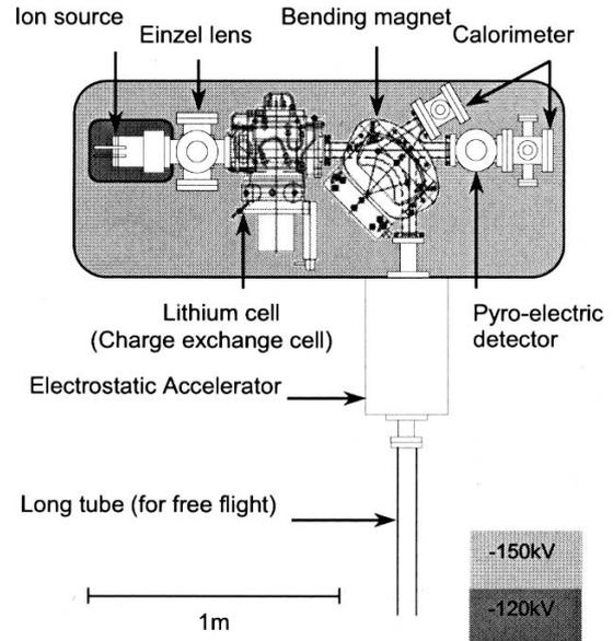
Fig. 2 Upper schematic diagram of the small sized test stand. The high voltage is applied in two stages. The one is applied a -150kV to extract He<sup>-</sup> beam by the electrostatic accelerator, the other is applied a -120 kV to extract He<sup>+</sup> beam from the ion source.
