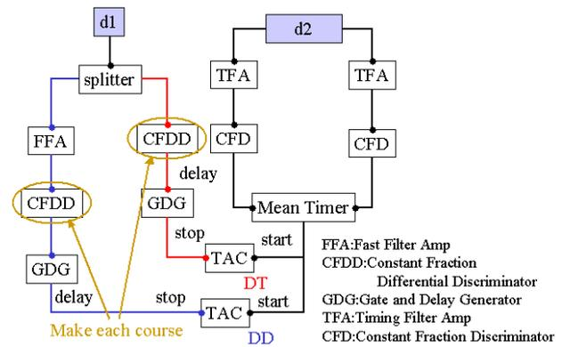
Fig. 4 The measurement system for neutron separation. The signal from d1 is divided into two routes using the splitter. The red line is DT neutron measurement route, and the blue line is DD neutron measurement route. Each route is made by CFDD.
