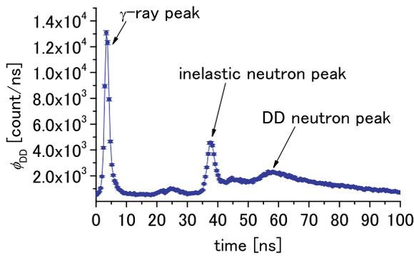
Fig. 5a The experimental result of neutron TOF spectrum separated from DT neutrons by fast discriminations of pulse heights in the d1 detector. The peak around 5 ns is  $\gamma$ -ray peak. The  $\gamma$ -ray peak originates in the inelastic scattering between  $^{12}\text{C}$  and DT neutron in d1. The peak around 38 ns is inelastic scattering neutron peak. The peak around 55 ns is DD neutron peak.
