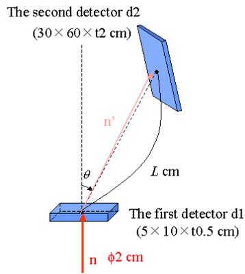
Fig. 3 MCNP calculation model for TOF spectrometer. This spectrometer has two plastic scintillators. The size of the fast detector is  $5 \times 10 \times 0.5$  cm, and that of the second detector is  $30 \times 60 \times 2$  cm. The considered parameter is  $\theta$ , and  $L$ .
