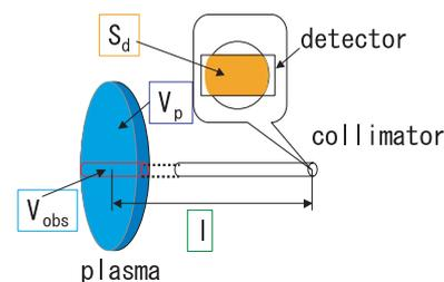
Fig. 1 The calculated ITER model.  $l$  is the distance between the center of the plasma and the measuring instrument.  $V_{\text{obs}}$  is plasma observation volume.  $S_d$  is the effective cross-section area
