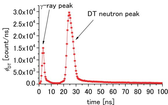
Fig. 5b The experimental result of neutron TOF spectrum separated from DD neutrons by fast discriminations of pulse heights in the d1 detector. The peak around 5 ns is  $\gamma$ -ray peak. The peak around 25 ns is DT neutron peak.
