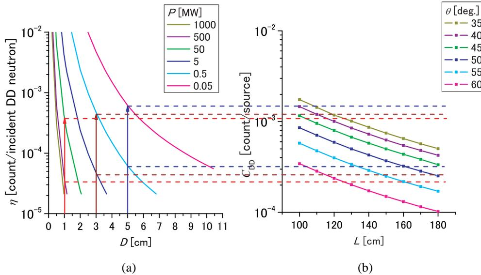
Fig. 2 (a) The tolerable lower limit of measurement efficiency against collimator diameter for every fusion power. (b) The measurement efficiency of TOF spectrometer designed using MCNP calculation. Some TOF spectrometer meet the requirement in the dynamic range from 0.05 to 1000 MW in fusion power by three collimators of 1 cm, 3 cm and 5 cm diameter, as indicated by arrows.
