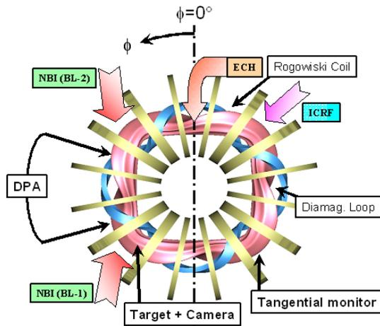
Fig. 1 Schematic view of the Heliotron J experimental setup.
