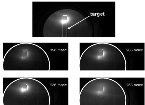
Fig. 5 Snapshots of the target image. The bright area corresponds to the hitting point of the diverted plasma. The white circle indicates the edge of the viewing port. (#23635)
