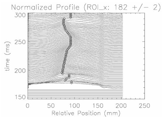
Fig. 6 The normalized profile of the brightness along the leading-edge for each time slice of the target image. (#23635)
