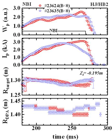
Fig. 7 Time traces of  $W_p$ ,  $I_p$ ,  $R_{\text{target}}$  and  $R_{\text{DPA}}$  for two NBI-only shots.
