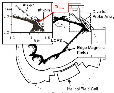
Fig. 2 Schematic view of the divertor probe array at  $\phi = 67.5^\circ$  with a Poincaré plot of the edge field lines. The inset shows the probe-pin positions.
