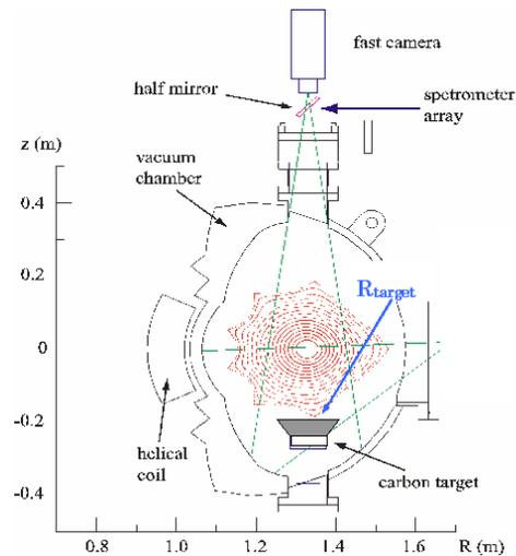
Fig. 3 Schematic view of the rail-limiter type carbon target and the fast-camera image monitoring system.
