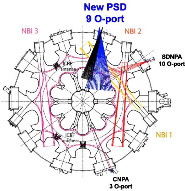
Fig. 1 Diagnostic location versus NBI and ICRF.
