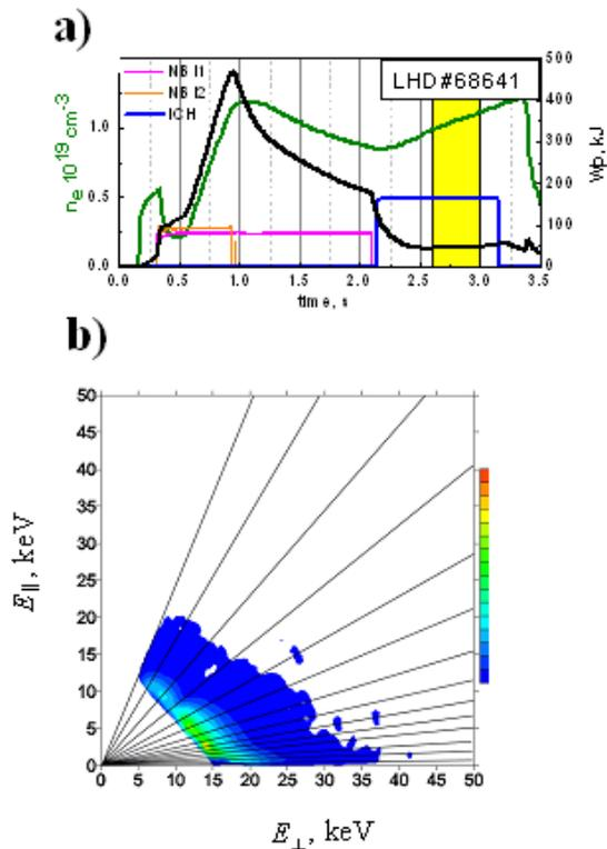
Fig. 7 (a) Time diagram of the LHD plasma discharge; (b) Restored proton angle and energy distribution calculated from PSD data for ICH-heated plasma.
