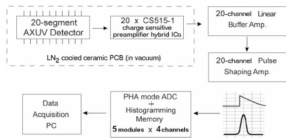
Fig. 4 Modified data acquisition system of the PSD.
