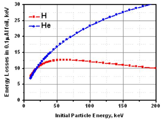
Fig. 3 Fast particles energy losses in 0.1 μ Al foil.
