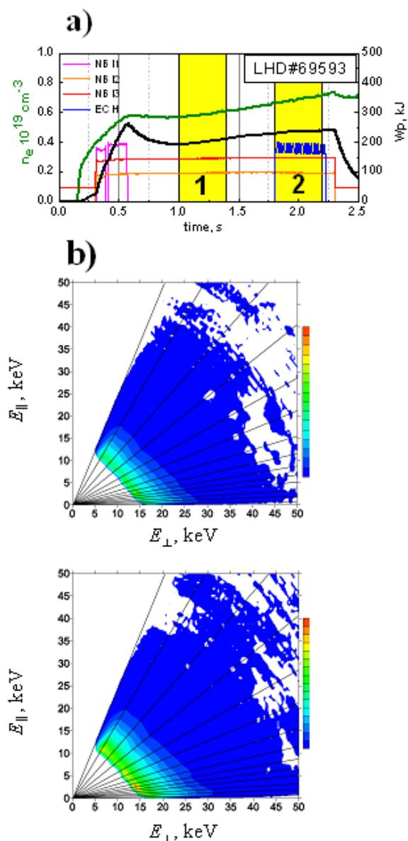
Fig. 6 (a) Time diagram of the LHD plasma discharge; (b) Restored proton angle and energy distribution calculated from PSD data: (1) for NBI-heated plasma and (2) for NBI- and ECH-heated plasma.
