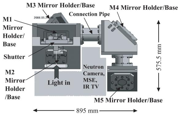
Fig. 3 Mechanical design of the front end optics in the equatorial port.
