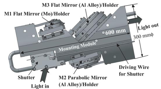
Fig. 2 Mechanical design of the front end optics in the upper port.
