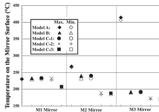
Fig. 4 Temperature on each mirror surface on the upper port calculated in the case of models tabled in Table 1 assuming the constant nuclear heating of 0.2 MW/m<sup>3</sup>.
