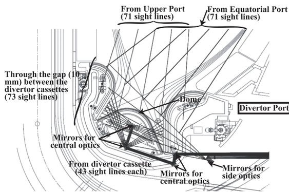
Fig. 1 Schematic view of the impurity influx monitor (Divertor) for ITER.
