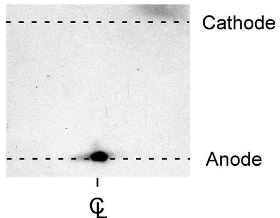
Fig. 4 X-ray pinhole photograph of the plasma exposed over 10 shots. The x-rays are generated at the center of the anode surface. The distance between the electrodes is 3 cm.
