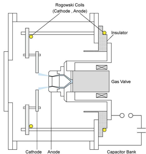
Fig. 1 Schematic diagram of the z-pinch device with divergent gas-puff. The ejection angle of the gas is  $10^\circ$  outward.
