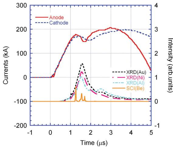
Fig. 2 Discharge currents, XRD and SCI signals of the divergent gas-puff z-pinch discharge.
