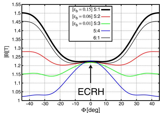
Fig. 1 Magnetic field on-axis of all the configurations used in the ECCD experiments.
