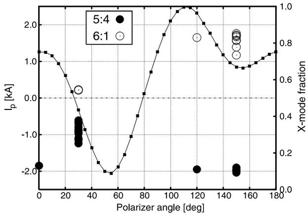
Fig. 2 Dependence of the total plasma current on the polarizer rotation angle and theoretical injected X-mode fraction in the 5:3 configuration (thin line with dots). Within the investigated values, the lower currents (either negative or positive) are observed when the fraction of power in the X-mode is around 0.3.
