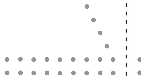
Fig. 4 Structure of horn antenna shown in Fig. 3, where the horn angle is 53.1 degrees. The photonic crystal is symmetrical with respect to the dashed line showing the waveguide center.
