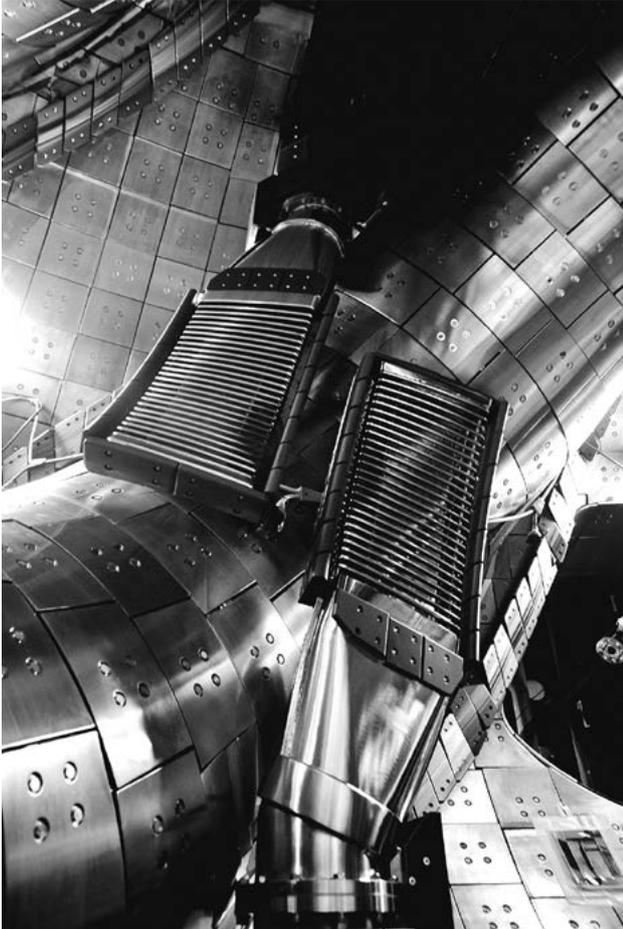
図6 Field-aligned ICRF antenna in the LHD.
