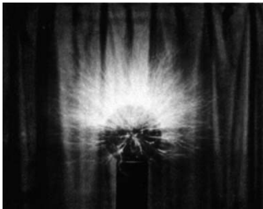
Fig. 13 Photograph of discharge from top of the Tesla coil high voltage generator.
