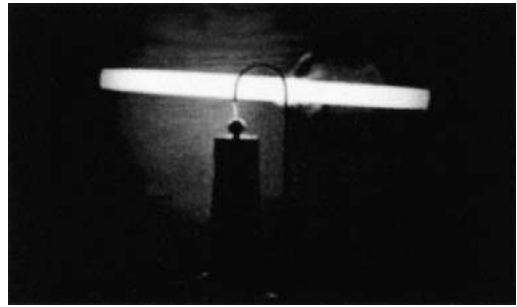
Fig. 14 Light emission from a non-connected fluorescent lamp excited with electromagnetic wave generated by Tesla coil.
