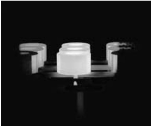
Fig. 6 Plasma electron annealing of gear blanks. The gear blanks are about 5 cm in dia. x 3 cm tall.
