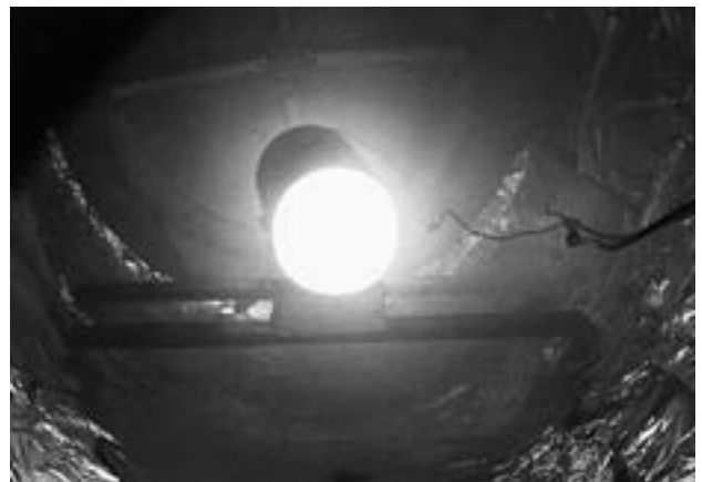
Fig. 7 Deposition of inner diameter of tubular structure using PBII & D technology. The tube size is about 5 cm in dia. x 30 cm long.
