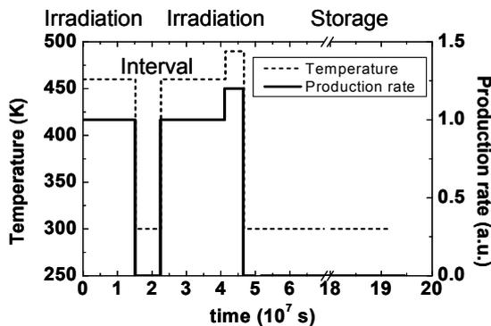
Fig. 3. Analytical conditions of the irradiation phase analysis. (H,T production rate and irradiation temperature during proton irradiation)
