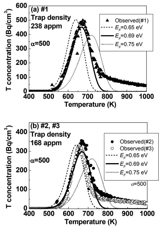
Fig. 8. Fitting results of the TDS analysis for the SS316 specimens using the trap site anneal model for  $\alpha=500$ . Where, (a) and (b) show the fitting results for #1 specimen and #2,3 specimens, respectively.
