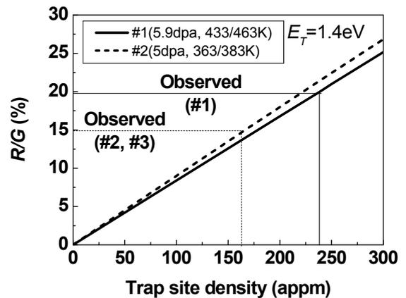
Fig. 5.  $R/G$  ratio in specimens for different trap site densities induced by the proton irradiation.
