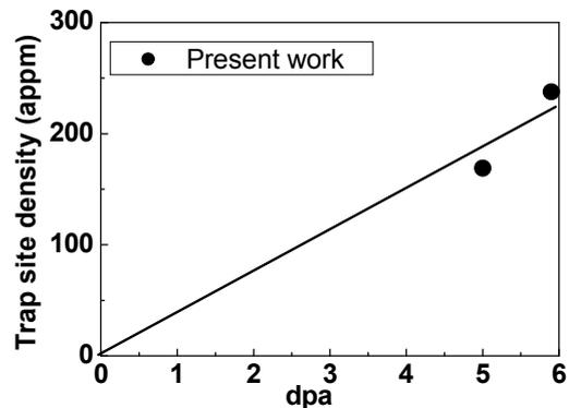
Fig. 6. Relationship between derived trap site density and irradiation dose by the irradiation phase analysis.
