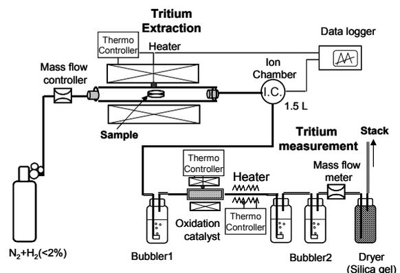
Fig.1. Schematic drawing of tritium measurement apparatus.
