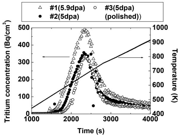
Fig.2. Tritium release behavior from the proton irradiated SS316 specimens (#1 ~ #3) (Ramp rate: 10 K/min., carrier gas: N<sub>2</sub>-2vol.%H<sub>2</sub>, flow rate: 250 cm<sup>3</sup>/min.)
