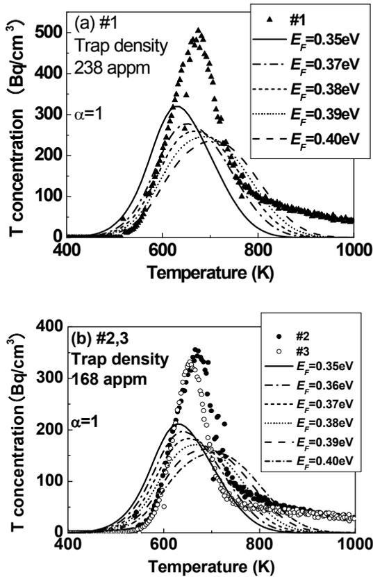
Fig. 7. Fitting results of the TDS analysis for the SS316 specimens using the trap site anneal model for  $\alpha=1$ . Where, (a) and (b) show the fitting results for #1 specimen and #2,3 specimens, respectively.
