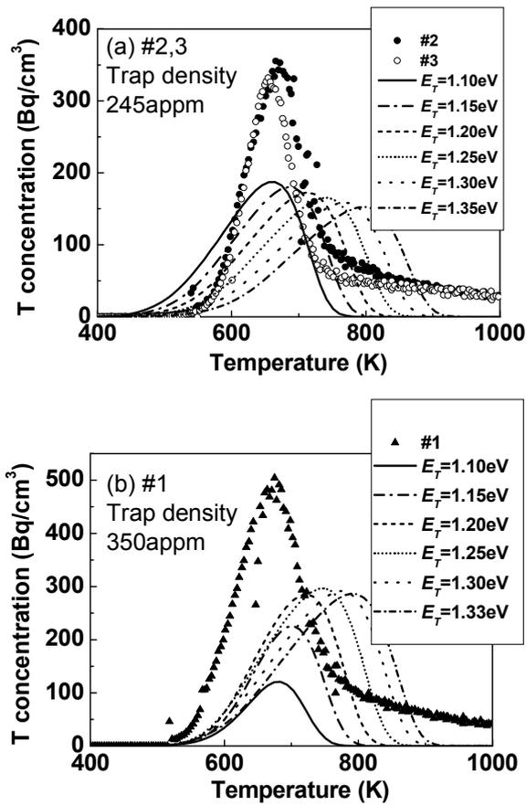
Fig. 4. Fitting results of the TDS analysis for the SS316 specimens using the de-trapping model. Where, (a) and (b) show the fitting results for #2, 3 specimen and #1 specimens, respectively.
