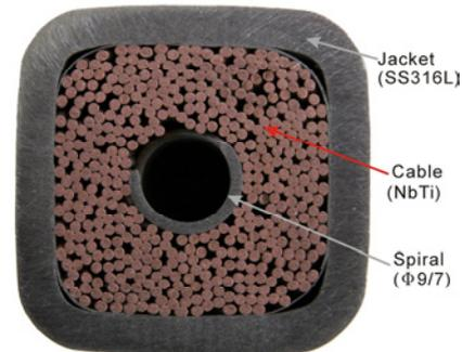
Fig. 7 EF-H conductor compacted from a circular tube
