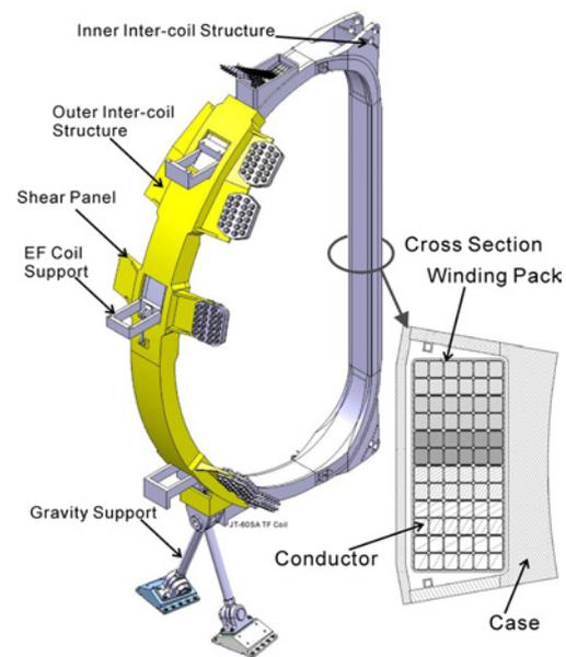
Fig. 3 TF coil with outer inter-coil structure
