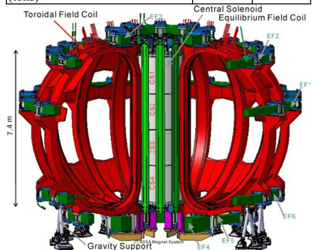
Fig. 2 Magnet system of the JT-60SA
