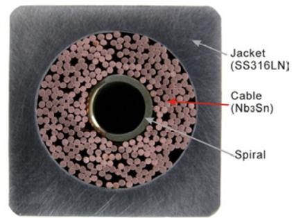
Fig. 6 CS conductor compacted from a round-in-square jacket
