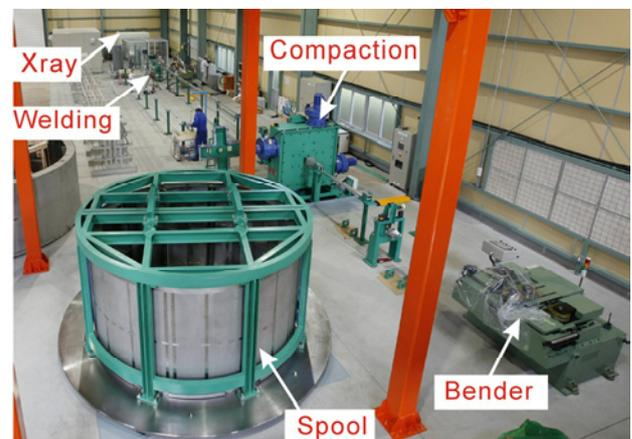
Fig. 9 Conductor assembly facility in Naka site
