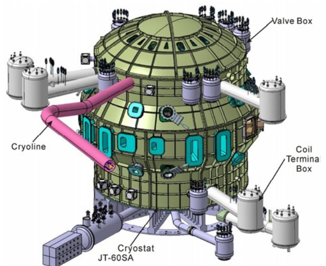
Fig. 8 Cryoline, valve box and coil terminal box
