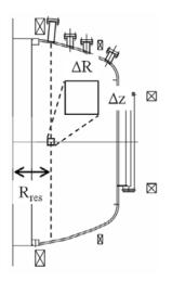
Fig.2 Volume in which we assume that electrons exist. In this study,  $\Delta R = \Delta Z = 0.005$ m and Rres = 0.19m. Hence, V has a cylindrical shape which has 0.19m inner radius, 0.005m thickness and 0.005m height.
