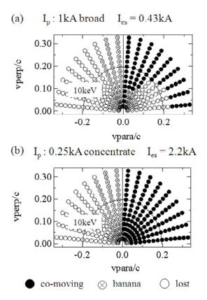
Fig.7 Improvement of confinement condition by the plasma current. The meaning of symbols is shown in the caption of Fig.5. Figure (a) shows the case in which 1kA plasma current distributes in broad area and figure (b) shows the case of concentration plasma current of 0.25kA.
