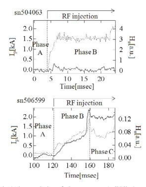
Fig.4 Time evolution of plasma current (solid line) and H $\alpha$  (dashed line). RF power in sn504063 is 70kW and in sn506599 is 50kW. B<sub>p</sub> in sn504063 is 120 Gauss and in 506599 is 40 Gauss.
