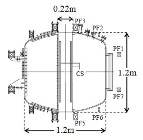
Fig.3 Side view of CPD including PF coils
