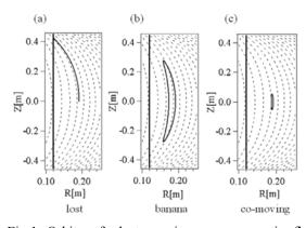
Fig.1 Orbits of electrons in open magnetic flux configuration. Solid lines show orbits projection, and dashed lines show magnetic line projection on poloidal plane.
