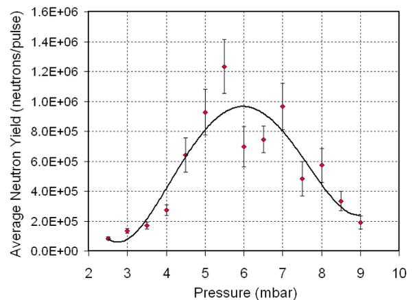
Fig. 4 Experimentally measured values of neutron yield as a function of D<sub>2</sub> filling gas pressure
