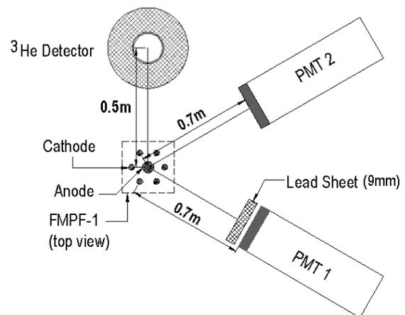
Fig. 2 Implemented diagnostics setup
