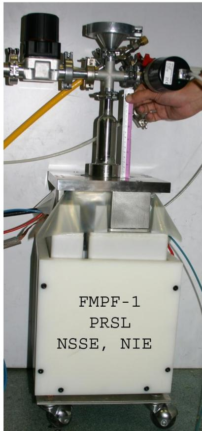
Fig.1 The 'FMPF-1' Miniature PF Device.
