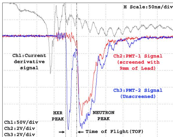
Fig. 3 Current derivative signal trace with HXR/neutron signals at 5mbar operating gas pressure.
